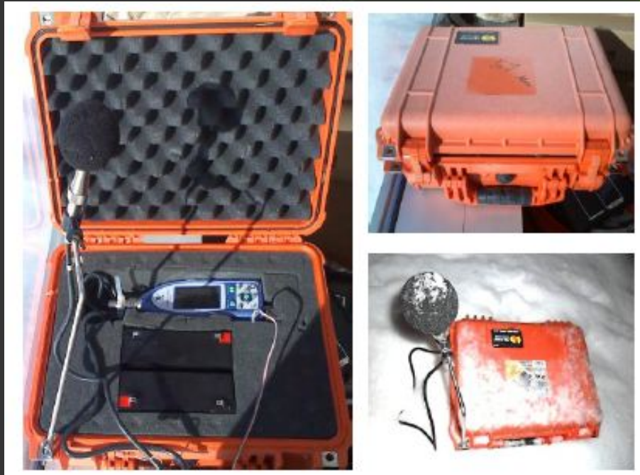
Example of configuration conducive for Sound-Level Meter Acoustical Counters.
