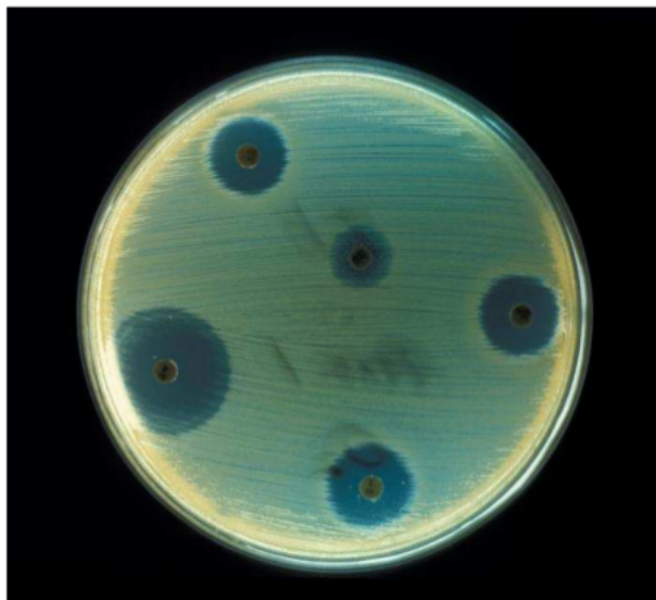
Figure 1.2. Example of the DIA test. The agar plate has several different drug disks. The clear zone around each of the disks is the test result. 2
