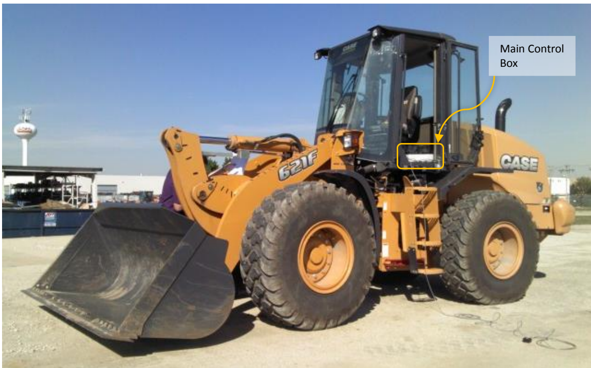
Fig. 69: External picture of the instrumented experimental wheel loader used within this research.
