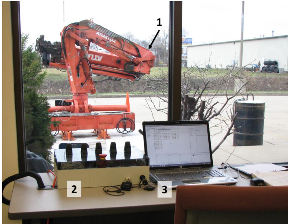
Fig. 35: Picture of the experimental crane from the measurement room of the Maha Fluid Power Research Center (Purdue University). The crane can be controlled from the portable control enclosure (2). The laptop (3) can be used to configure the control unit e perform real-time acquisition. The point 1 indicates the location of the outer boom accelerometer.
