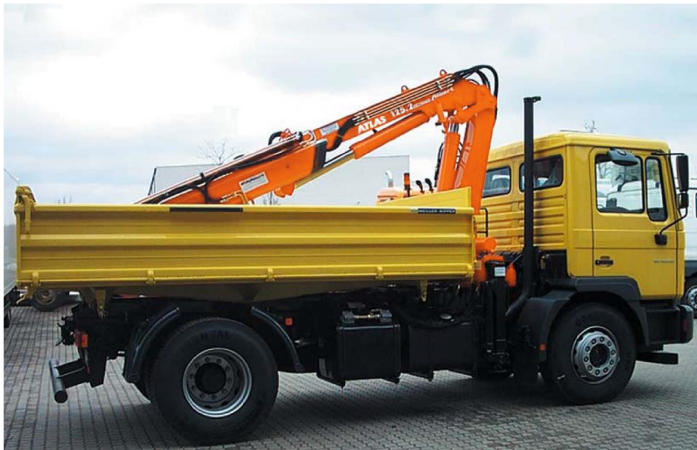
Fig. 33: Truck mounting of the reference crane from manufacturer documentation (Atlas Maschinen Gmnh®, 1996).
