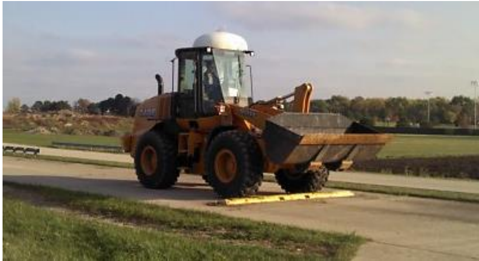
Fig. 91: Picture of the experimental wheel loader driving on the bump test track located at the research sponsor facility.
