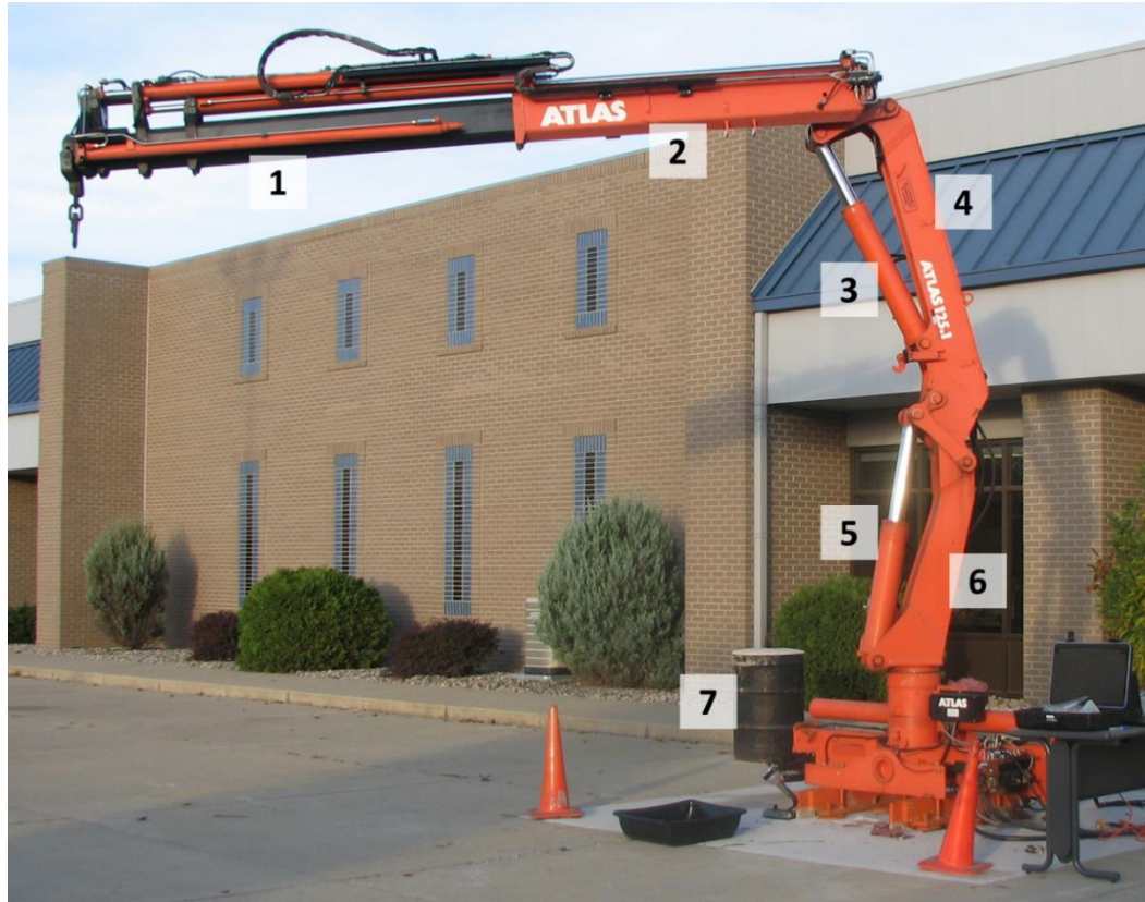
Fig. 34: Picture of the experimental crane installed at Maha Fluid Power Research Center (Purdue University): 1) telescopic stages; 2) telescopic boom; 3) telescopic boom actuator; 4) outer boom; 5) outer boom actuator; 6) main boom; 7) load (barrel of concrete, 1000kg).
