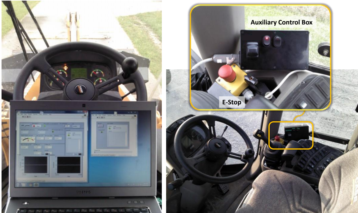
Fig. 70: Internal picture of the instrumented experimental wheel loader used within this research.
