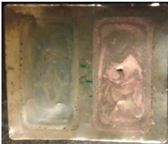
Figure 9.5 A LIAD foil prepared using forming mandrels C2 in the drying gas chamber. Brilliant green was deposited on the left side of the foil and octaethyl porphyrin was deposited on the right side (reproduced from Reference 10).
