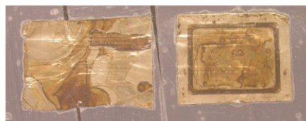
Figure 7. (Left) A LIAD foil with asphaltene deposited on it by using the dry-drop technique, showing that the analyte layer is very uneven, with spots of heavy sample amounts and areas of little to no sample. (Right) A LIAD foil with asphaltene deposited on it by using the drying gas chamber, showing that the surface is more uniform than for the dry-drop method.
