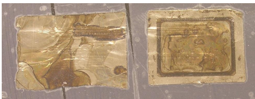
Figure 9.3 Comparison of a LIAD foil with asphaltenes deposited on it by using the dry drop method (left) and a LIAD foil with asphaltenes deposited on it by using the drying gas chamber (right). A visual comparison of the two samples indicates that the sample is deposited much more uniformly using the drying gas chamber (reproduced from Reference 10).
