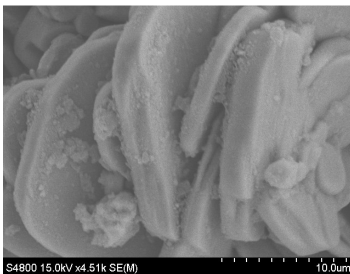
Figure D.1. Scanning electron image (SEM) of Calcium Cobalt Oxide (Ca 3 Co 4 O 9 ).
