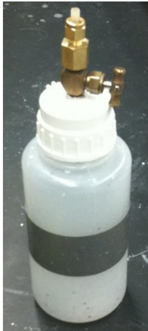
Figure 2.9 A valve was fitted to a ball mill bottle to evacuate using a vacuum pump.
