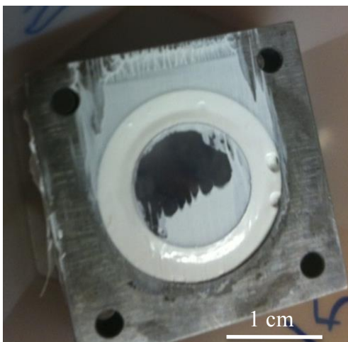
Figure 2.7 Ring-shaped mold with tapered Plexiglas centerpiece with formed alumina part immediately after injection molding.
