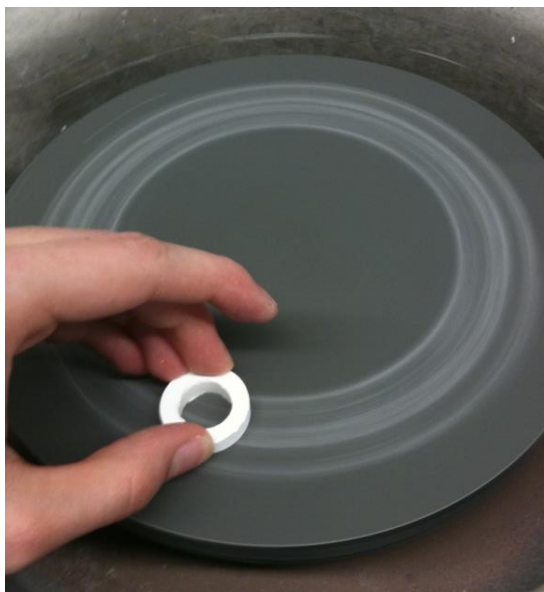
Figure 2.13 Evening out surfaces of an alumina ring in the green state using a polishing wheel.
