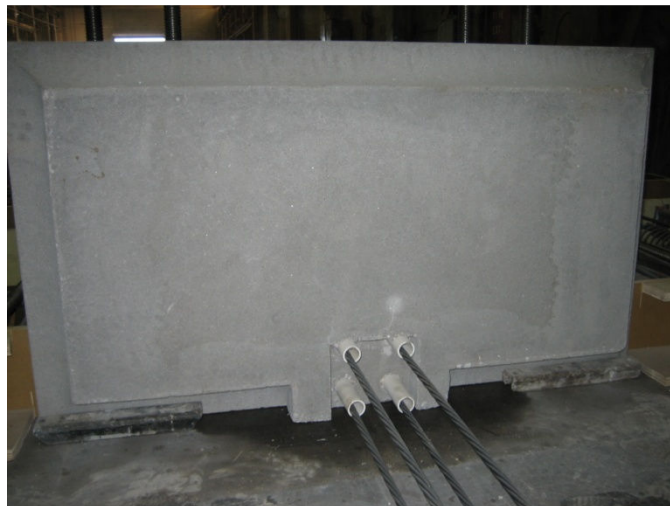
Figure 70 Exterior face of post with strands protruding.
