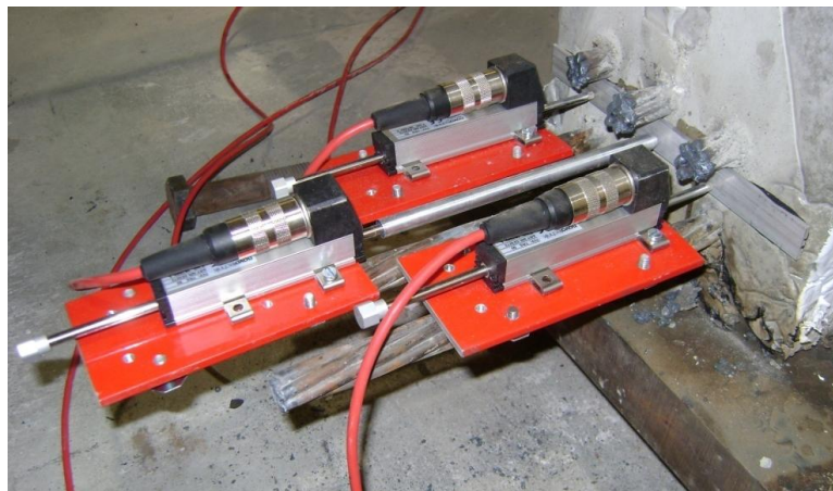
Figure 25 Potentiometers Attached to the Bottom Row of Strands
