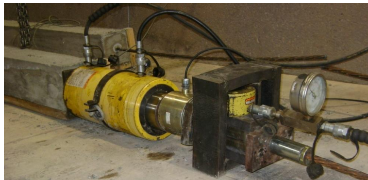
Figure 21 Pull-out Testing Setup
