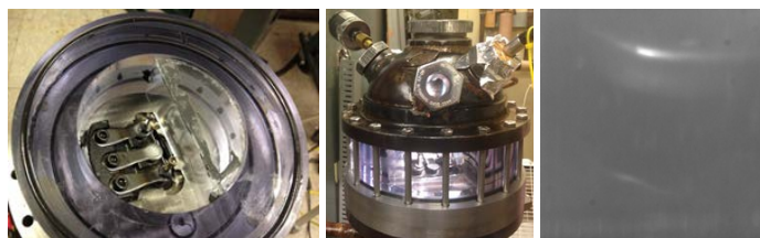
Figure 4: Visualization setup: transparent flange and glass barrier to enhance optical access to the valve and sample image for the valve vicinity.
