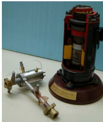
Figure 4: Comparison between the proof-of-concept turbocompressor and an equivalent scroll compressor.
