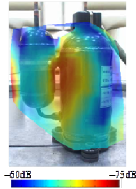
1.25-kHz band Figure 14: Sound Intensity Map of Original Compressor
