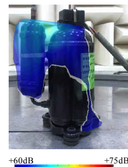
1.25-kHz band Figure 17: Sound intensity map of improved compressor
