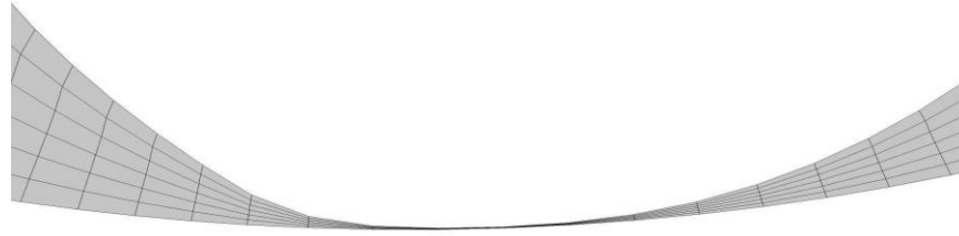
Figure 10: Mesh density in the tip gap area with 6 divisions in the radial direction
