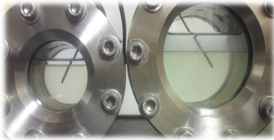
Figure 7: Partial miscibility of R-290/PAG3_ISO68 at 24°C (297.15 K), and absolute refrigerant concentration: 23% (left figure) and 31% (right figure)
