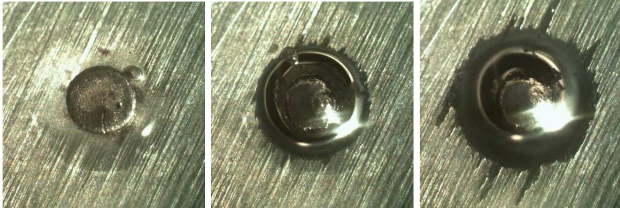
(a) filler metal disc on AA3003 plate (b) initial melting of the filler metal (c) extensive spreading of filler metal
