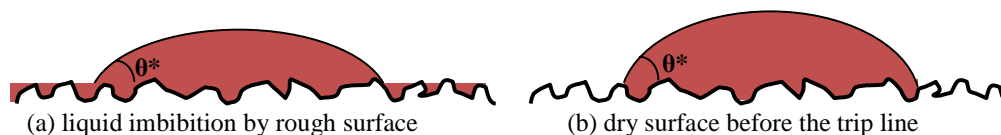
Figure 9: Illustration of apparent contact angle \theta^* on a rough surface (Bico et al., 2001)
