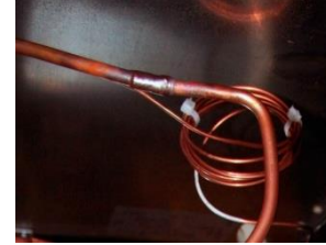
a) capillary tube inside suction line
