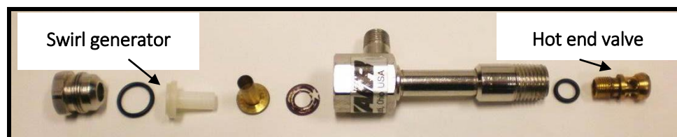
Figure 6: Vortex tube with its components
