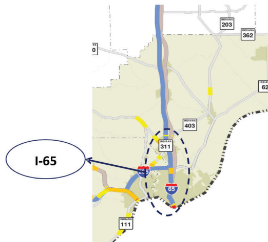
Figure 4.1 Map indicating LOS in the year 2010 on the six potential corridors considered for identification of a congested corridor for the simulation based analysis.
