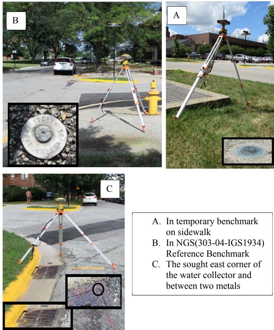
Figure A.9 Rapid Static Points Measured in Agriculture Mall at Purdue University Campus to check RTK GPS System accuracy
