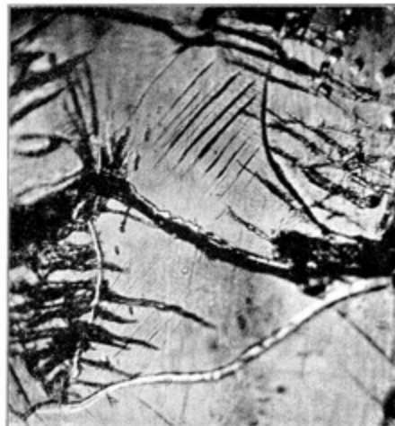
Figure 1. Formation of slip bands in steel as captured by Ewing and Humfrey in 1903 [8] .
