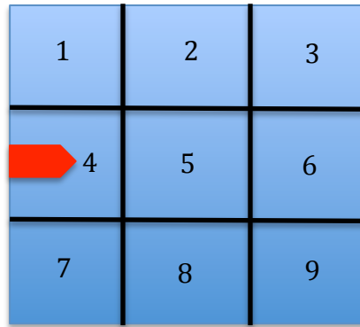
Figure 53. Diagram detailing the arrangement of the nine images captured at each load level. The red area represents the crack tip.
