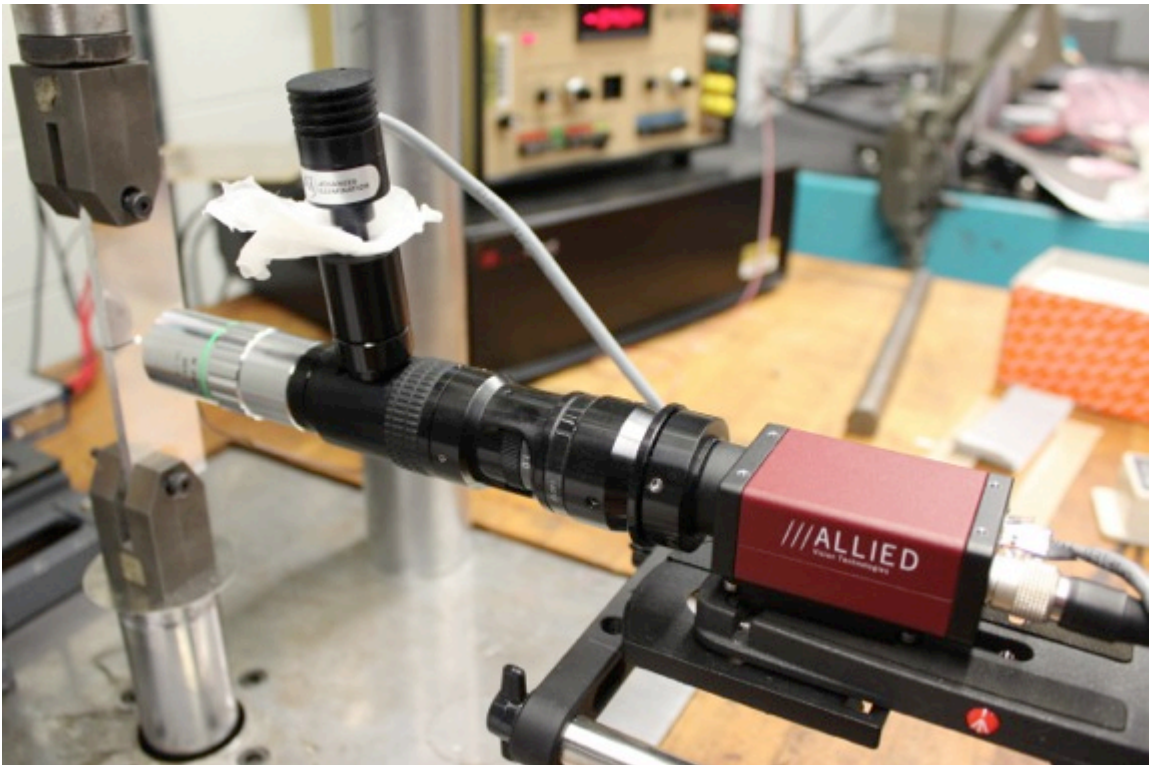
Figure 18. Allied Vision Technologies Manta 210 camera setup.
