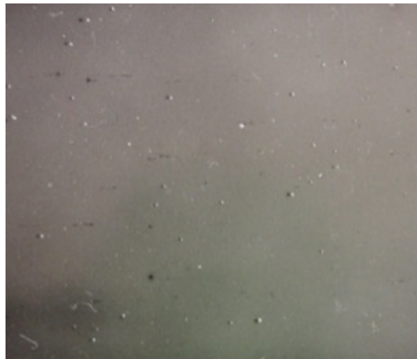
Figure 25. Clumping of silica particles on the material surface.
