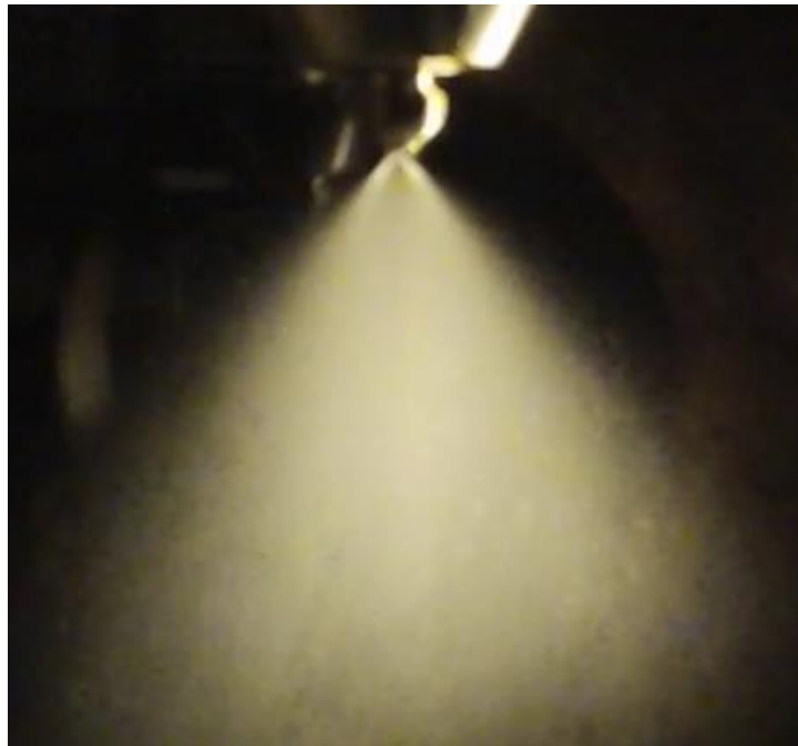
Figure 3.10. Spray Visualization of Super Atmospheric Testing Pressure Swirl Injector, JP-8, 0.172 MPa (25 psi) Ambient Pressure.
