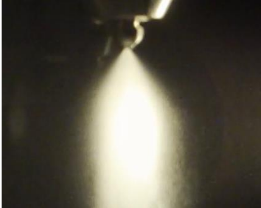
Figure 3.11. Spray Visualization of Super Atmospheric Testing Pressure Swirl Injector, JP-8, 1.723 MPa (250 psi) Ambient Pressure.
