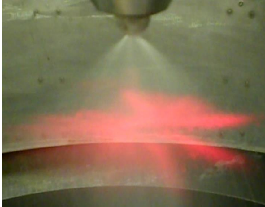
Figure 3.9. Spray Visualization of Optical Patternator Pressure Swirl Injector, JP-8, -40 C Fuel Injection Temperature.
