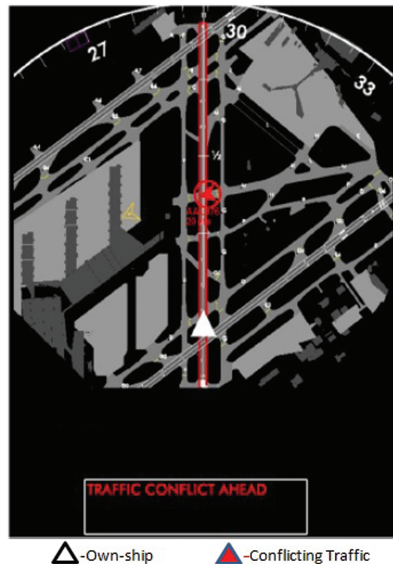
Figure 1. Conceptual cockpit display of a Warning alert from SURF-IA. Adapted from "Safety, Performance and Interoperability Requirements Document for Enhanced Traffic Situational Awareness on the Airport Surface with Indications and Alerts (SURF-IA)," by Radio Technical Commission for Aeronautics (RTCA/DO-323).
