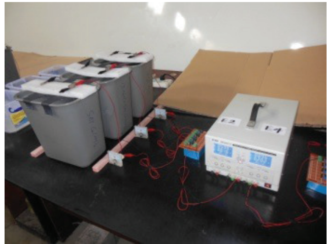
Figure 4. Test setup of simulated ICCP systems.
