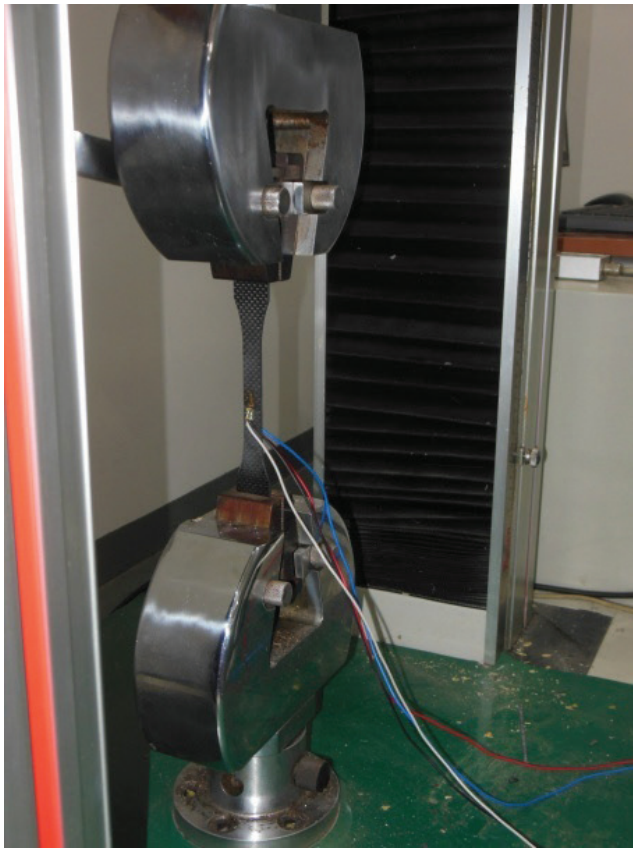
Figure 5. Test rig for tensile tests.
