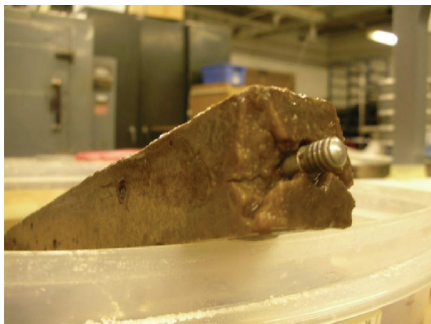
Figure 9. The loosened stud in mortar bar with Ottawa sand after 146 days of storage in the 25 wt% \text{MgCl}_2 solution.
