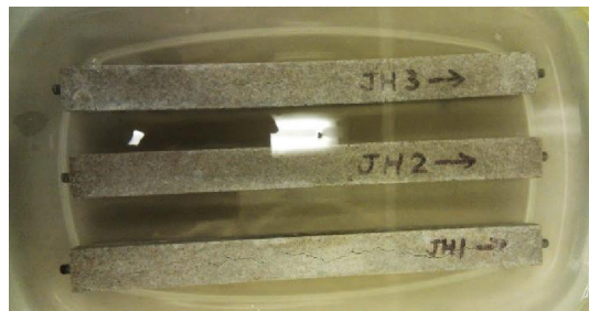
Figure 1. Mortar bars with Jobes and in the NaOH soak solution.
