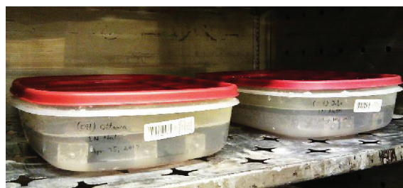
Figure 2. Mortar bars in the sealed containers in the 80°C oven.
