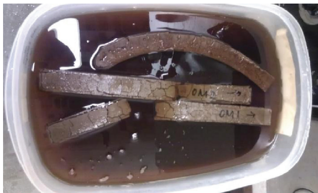
Figure 10. Cracking and bending of mortar bars with Ottawa sand after 257 days of storage in the 25 wt% \text{MgCl}_2 solution.
