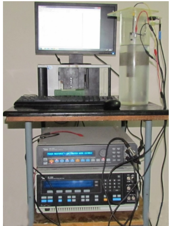
Figure 4. Corrosion test setup with corrosion cell, potentiostat, and computer.
