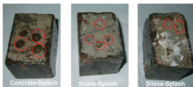
Figure 6. Silane concrete conditions of hydrophobic nature after 5 years' exposure age.
