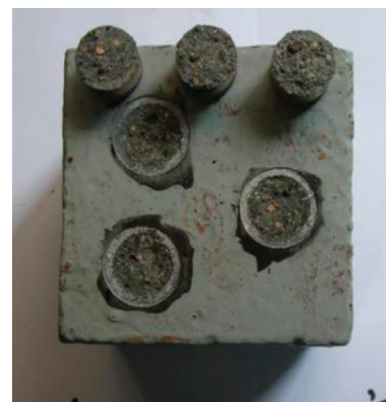
Figure 5. Typical damage type of concrete coating.
