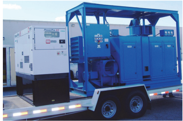
Figure 2. Trailer-mounted desiccant dehumidifier
