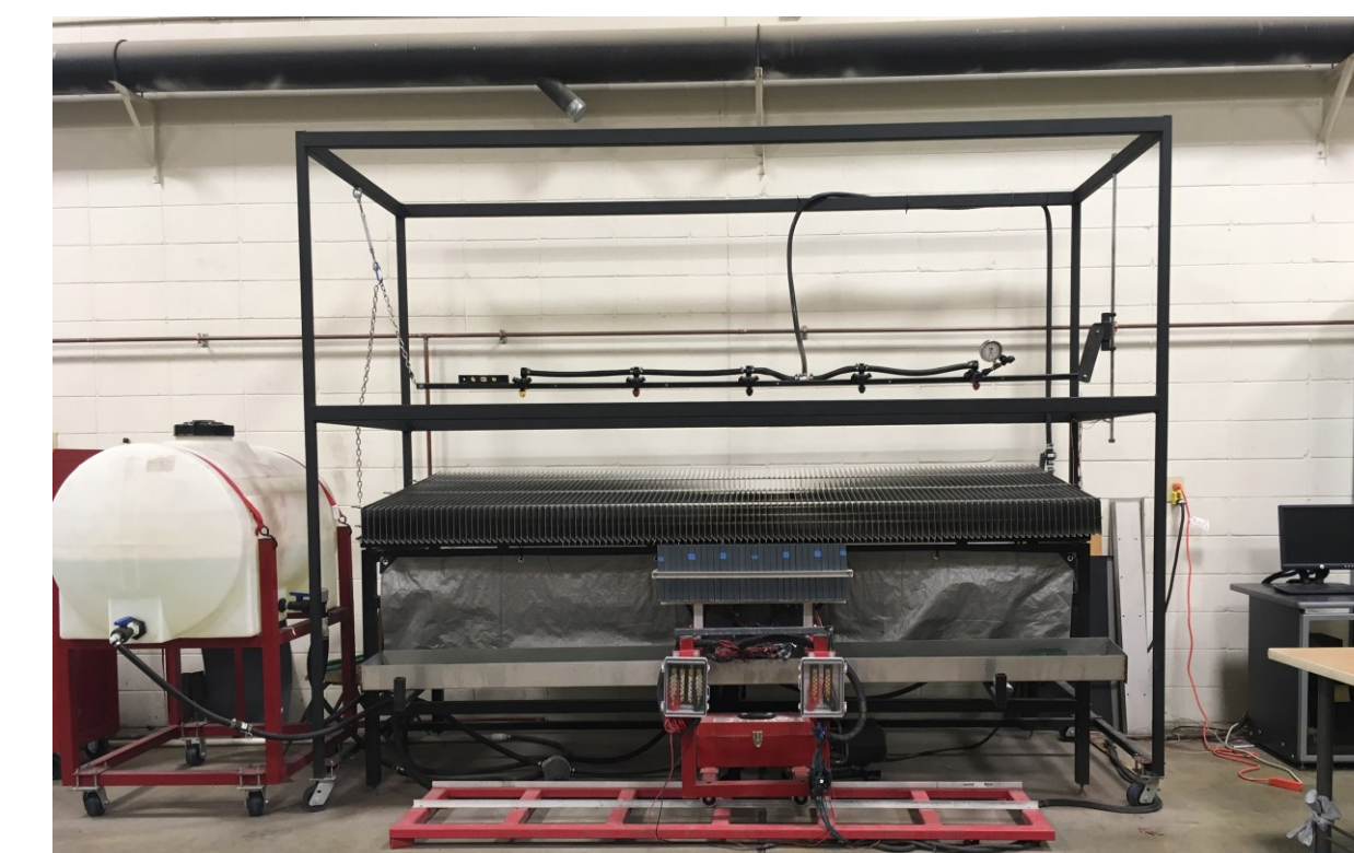
Figure 2: Laboratory Spray Application Simulator.
