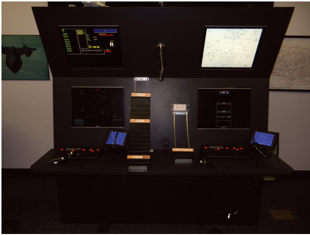
Figure 1. Each en route air traffic control simulation system is composed of two positions, a radar side (R-side) on the left and a data side (D-side) on the right. Participants in this study worked in the R-side position. During the nonradar condition, they were supported by an assistant in the D-side position.
