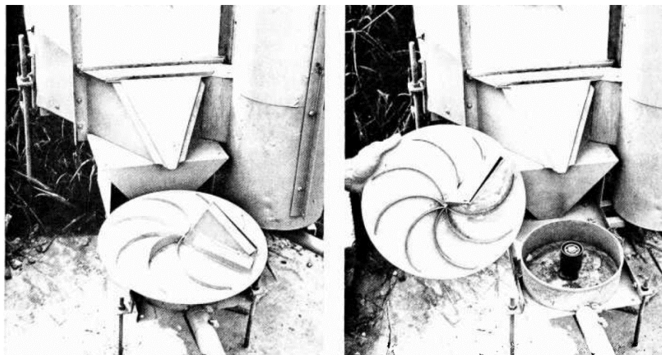
Figure 2-23 Rotational flow sampler completely assembled (left) and with wheel removed (right) (Brakensiek et al. 1979)
