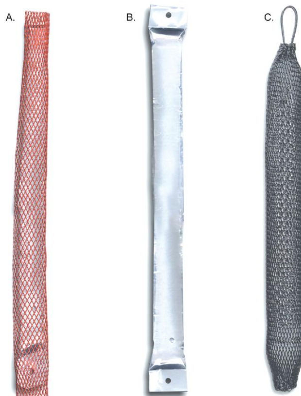
Figure 2-8 Passive diffusion bag sampler (b) with protective mesh (a) & (c) (Vrobley 2001a)
