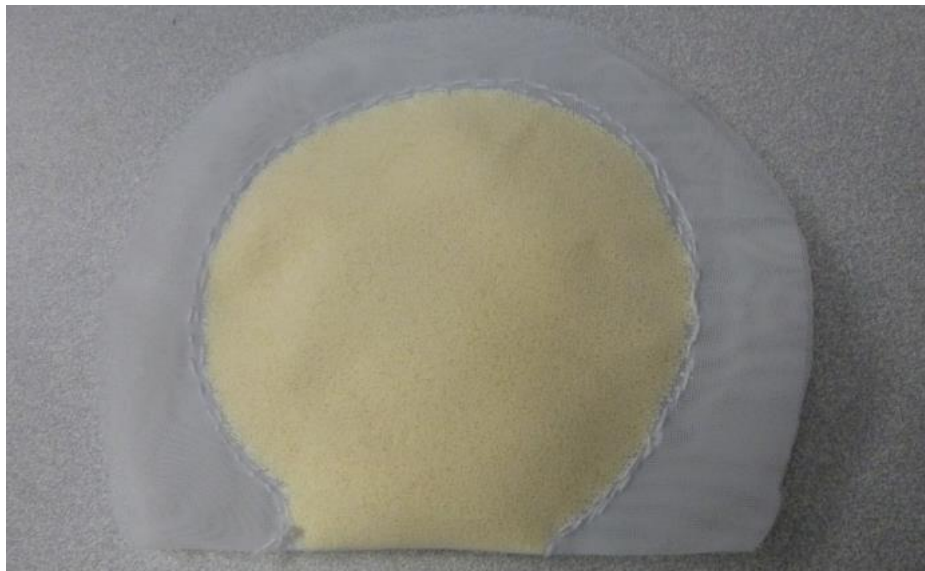
Figure 4-24 Ion exchange resin sampler used in supplemental tests. The sampler's dimensions were the same as the housing units and BMP columns to ensure all the synthetic stormwater flowing through the sampler
