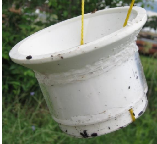
Figure 4-13 Bioretention deployment unit influent sampler housing
