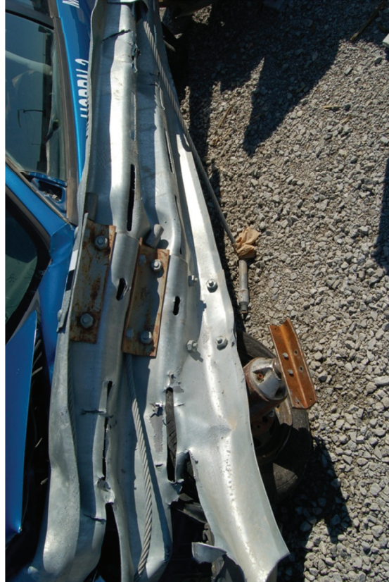
Figure 42. System Damage, Test No. USPB-N-3
