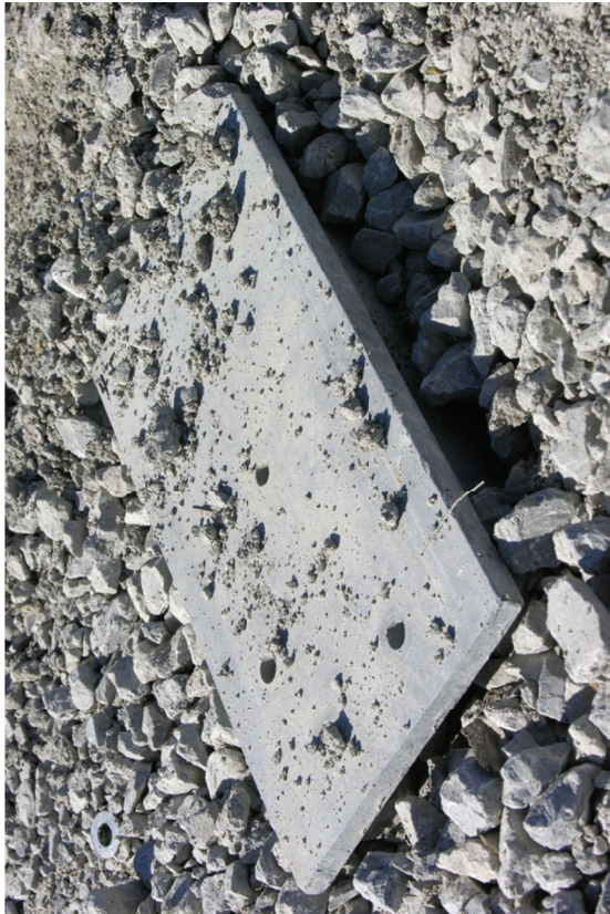
Figure 53. Post Damage, Test No. USPBN-4
