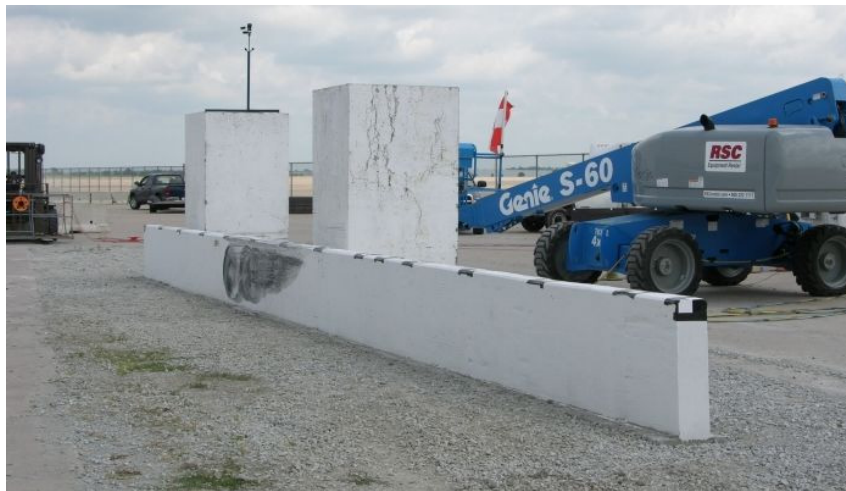
Figure 18. System Damage, Test CBPP-1
