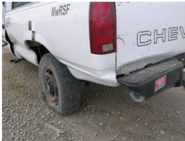
Figure 29. Vehicle Damage, Rear of Vehicle, Test CBPP-1
