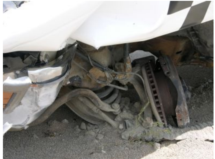
Figure 24. Vehicle Damage, Left-Front Wheel, Test CBPP-1
