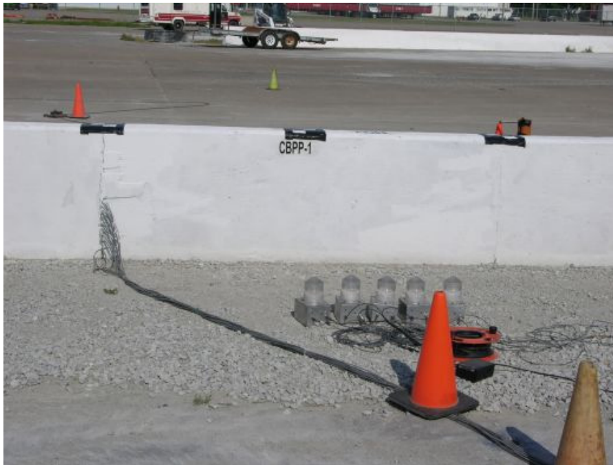
Figure 6. Backside Test Installation and Strain Gauge Wires, Test CBPP-1
