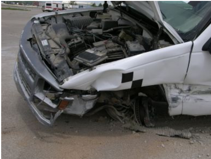
Figure 24. Vehicle Damage, Left-Front Wheel, Test CBPP-1
