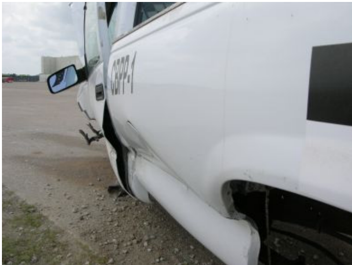
Figure 25. Vehicle Damage, Left Side, Test CBPP-1
