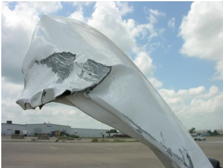
Figure 27. Vehicle Damage, Hood and Windshield, Test CBPP-1
