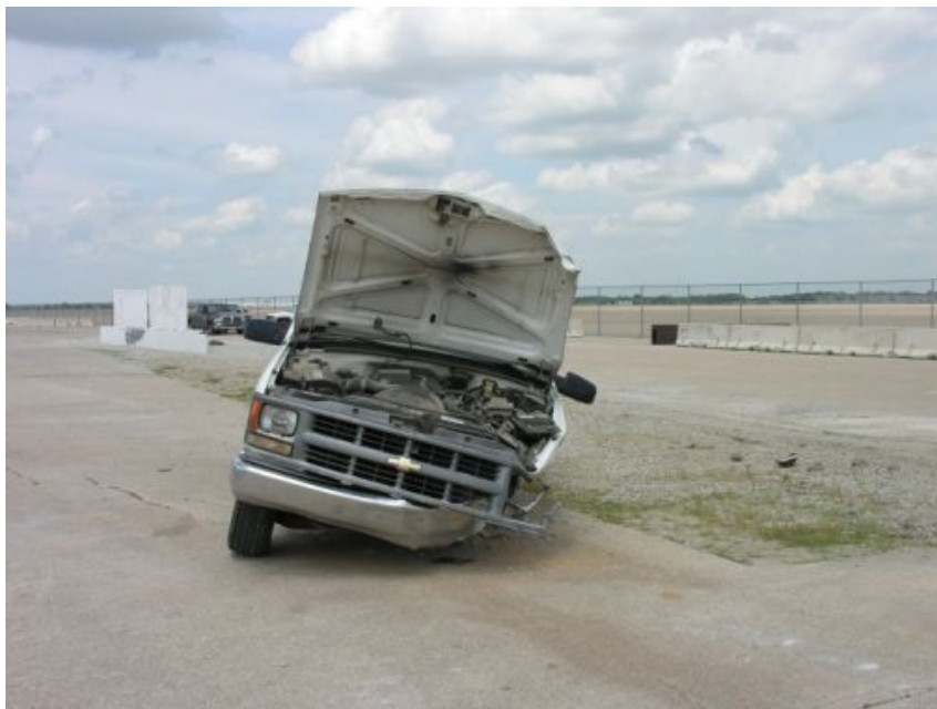
Figure 17. Vehicle Final Position and Trajectory Marks, Test CBPP-1
