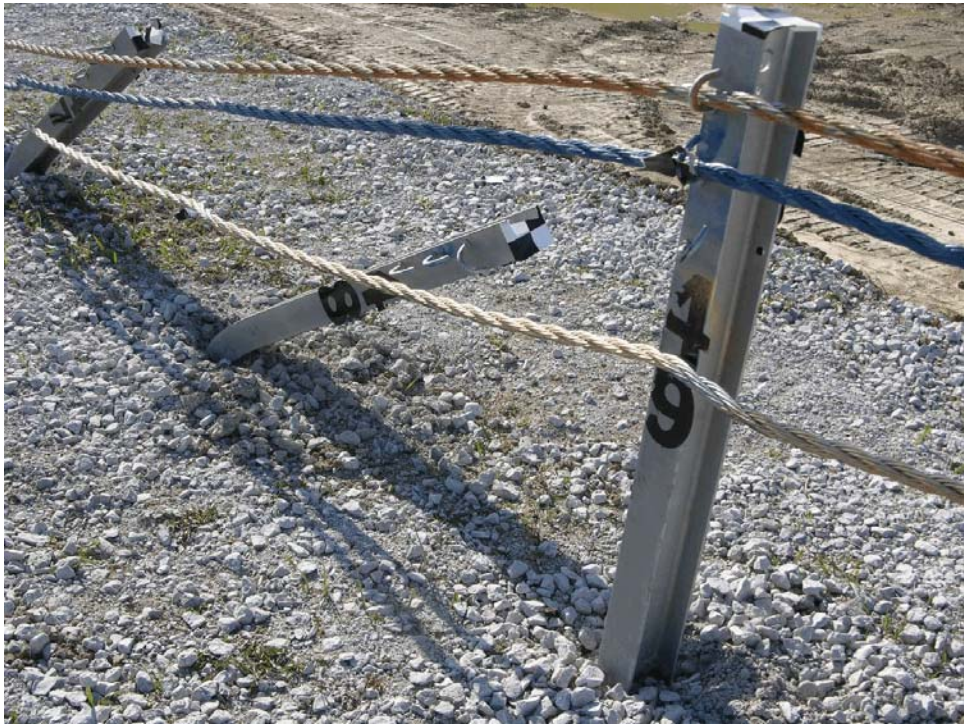
Figure 33. System Damage, Test CS-2
