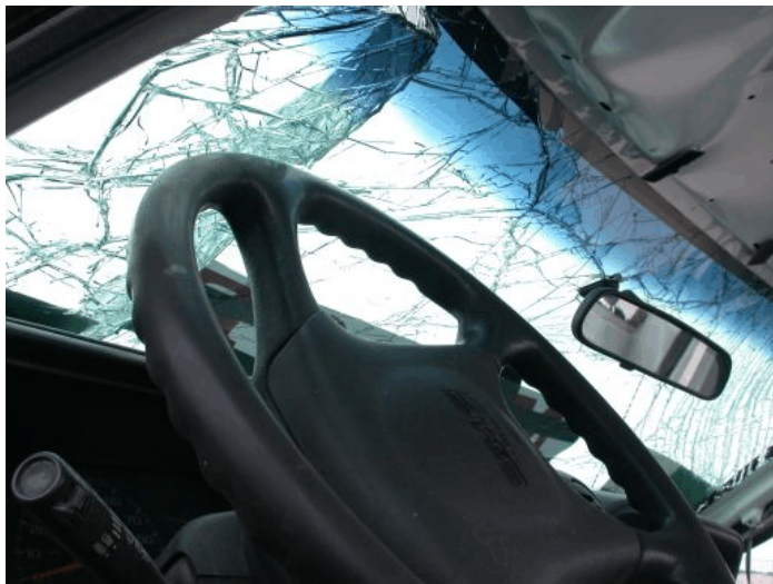
Figure 49. Occupant Compartment and Windshield Damage, Test MWT-3
