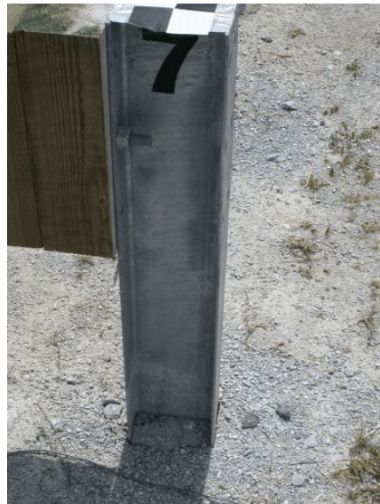
Figure 74. Post Nos. 7 through 9 Damage, Test MWT-4
