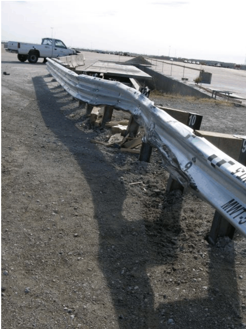
Figure 106. System Damage, Test MWT-5
