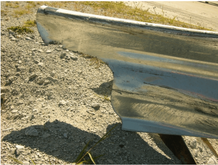
Figure 72. Rail Rupture Damage, Test MWT-4
