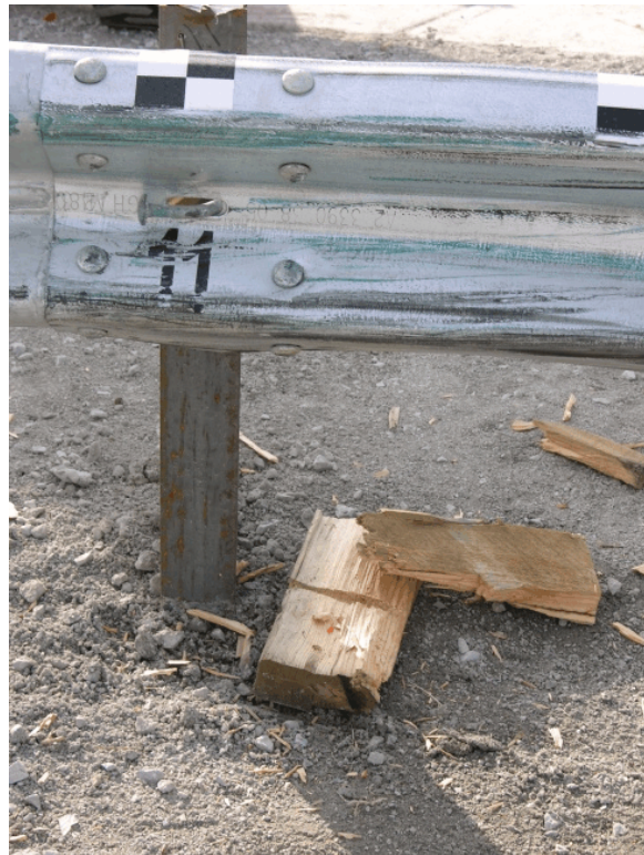
Figure 126. Post Nos. 10 and 11 Damage, Test MWT-6
