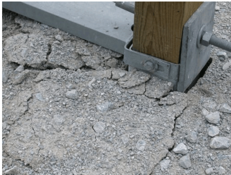
Figure 41. Anchorage Damage, Test MWT-3
