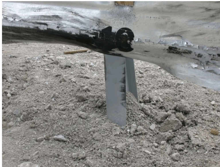
Figure 42. Post Nos. 9 and 10 Damage, Test MWT-3
