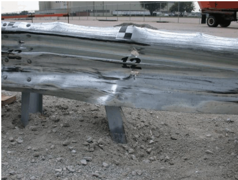
Figure 43. Post Nos. 11 and 12 Damage, Test MWT-3
