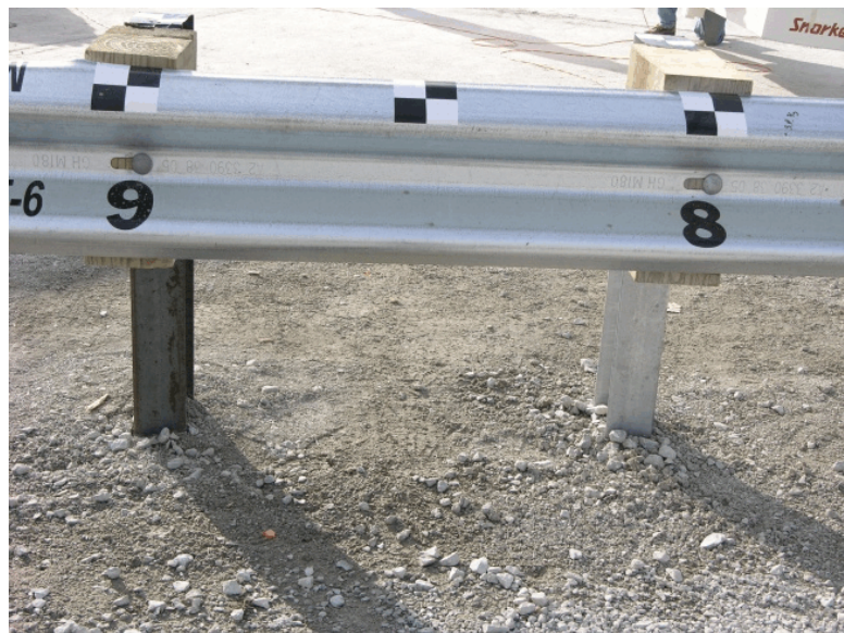
Figure 125. Post Nos. 6 through 9 Damage, Test MWT-6
