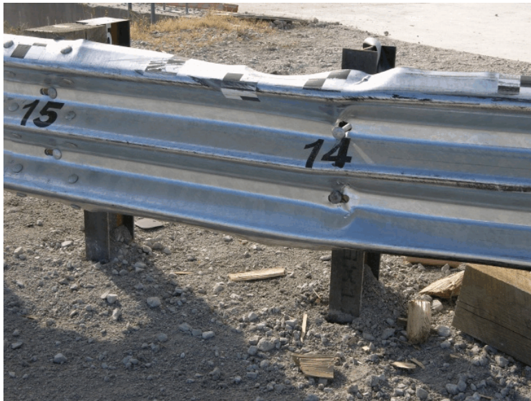
Figure 111. Post Nos. 13 through 16 Damage, Test MWT-5
