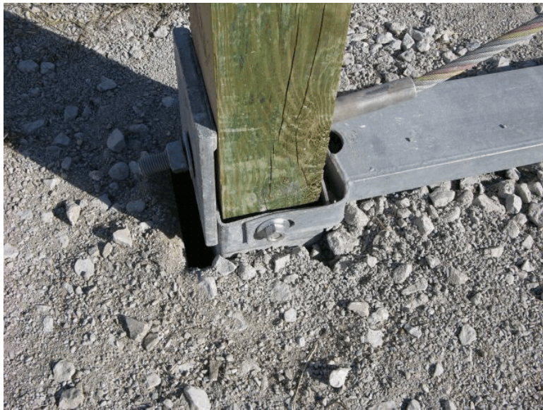
Figure 107. Anchorage System Damage, Test MWT-5
