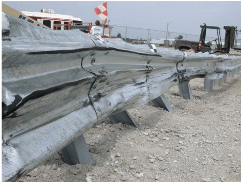
Figure 40. System Damage, Test MWT-3
