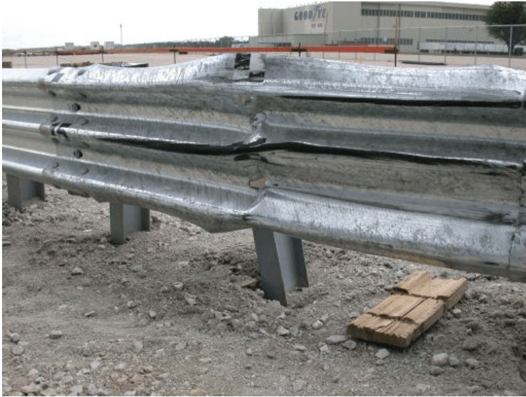
Figure 44. Post Nos. 13 and 14 Damage, Test MWT-3
