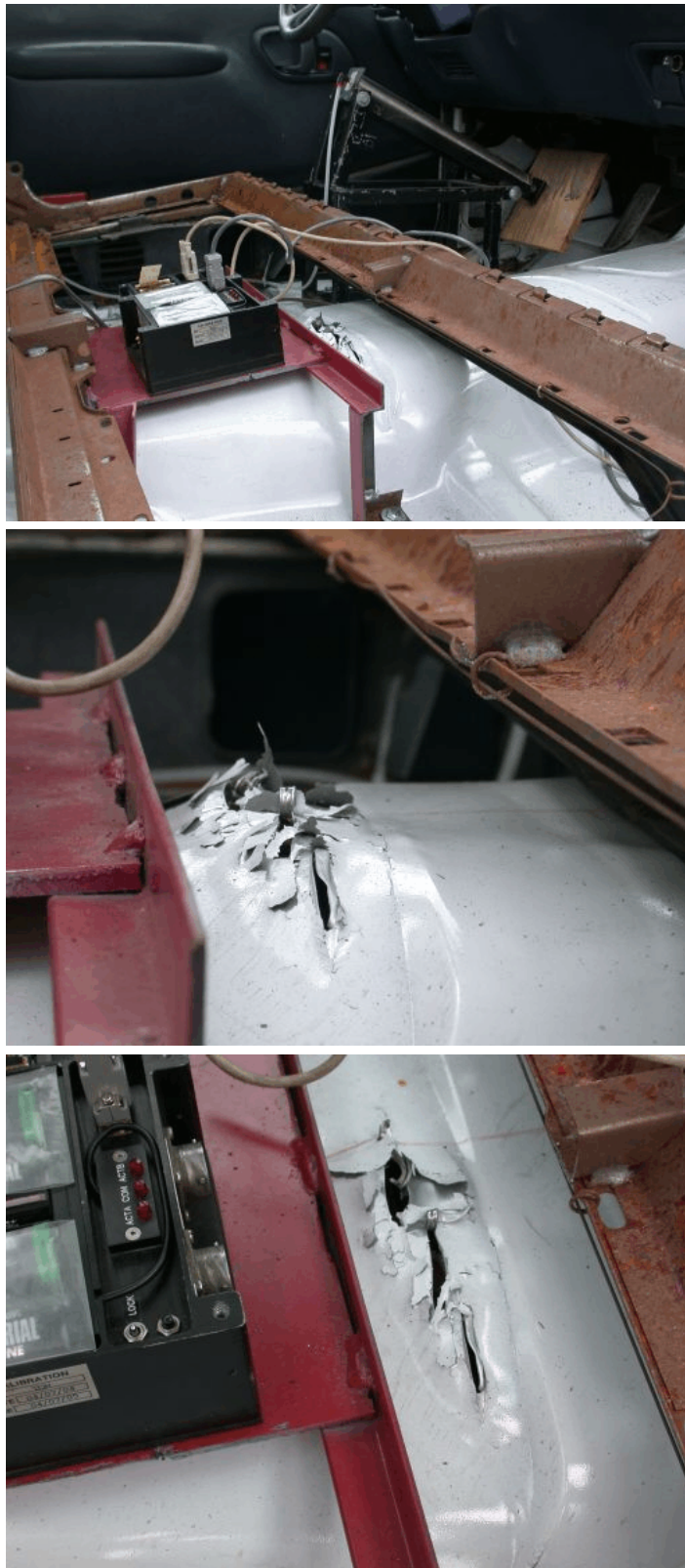
Figure 80. Occupant Compartment Damage, Test MWT-4
