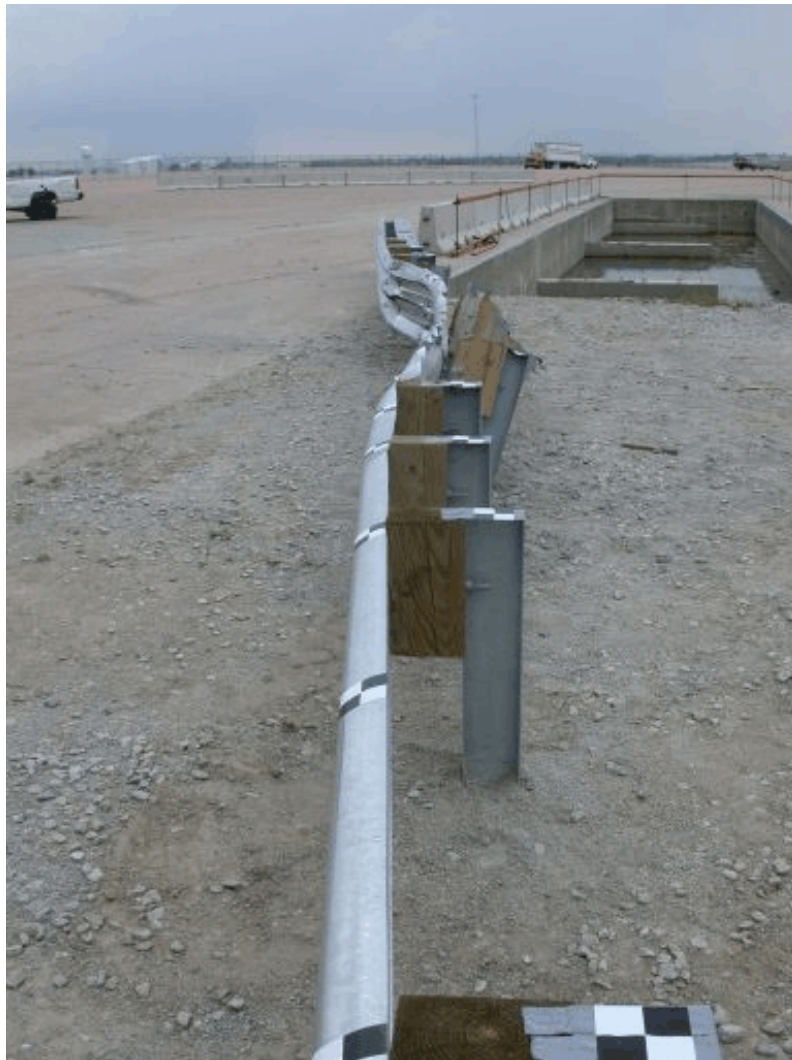
Figure 39. System Damage, Test MWT-3
