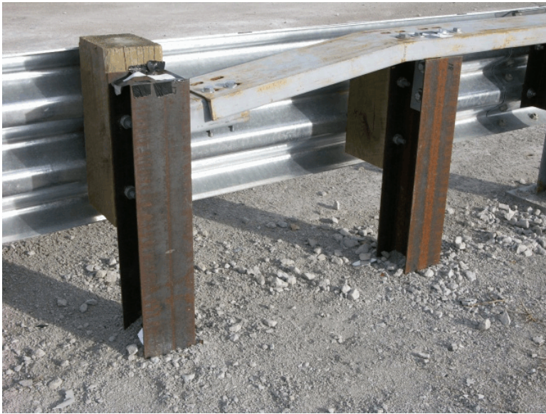
Figure 128. Post Nos. 14 through 19 Damage, Test MWT-6
