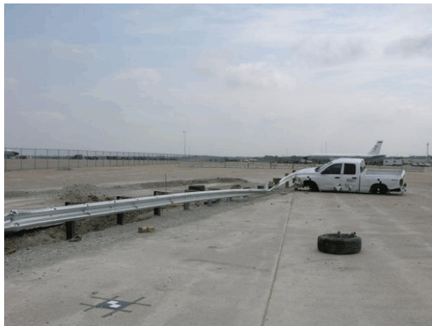
Figure 32. Vehicle Final Position and Trajectory Marks, Test No. MGS221-1
