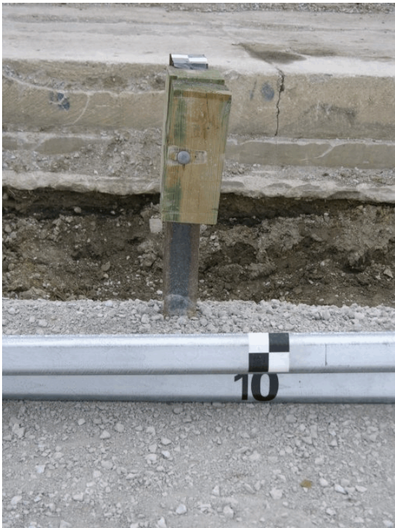
Figure 60. Post Nos. 9 through 12 Damage, Test No. MGS221-2
