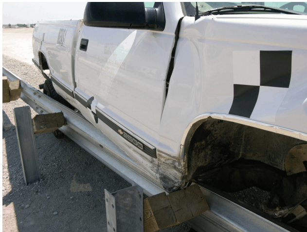
Figure 34. Vehicle Damage, Test No. MGSAS-1
