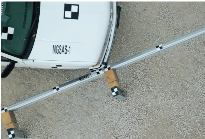
Figure 25. Impact Location, Test No. MGSAS-1
