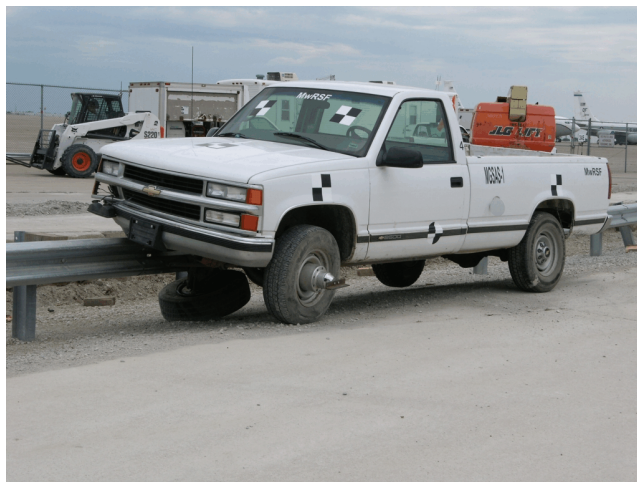
Figure 33. Vehicle Damage, Test No. MGSAS-1
