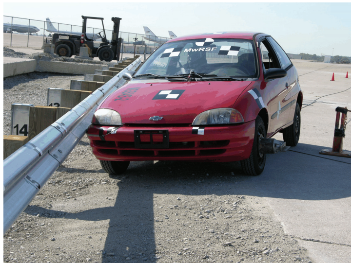
Figure 41. Impact Location, Test No. MGSAS-2
