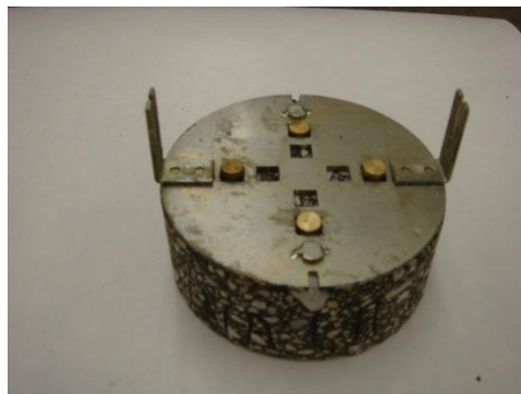
Figure 3.21 Gauge-point mounting device
