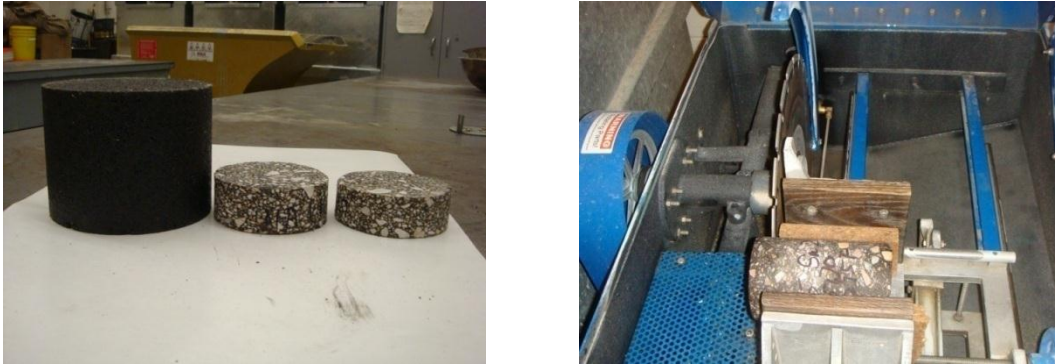
Figure 3.20 Testing specimens after coring-sawing process
