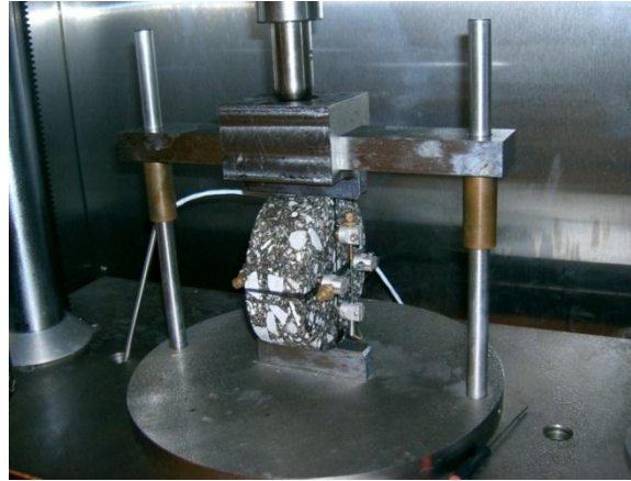
Figure 3.22 An IDT specimen installed in the UTM-25kN
