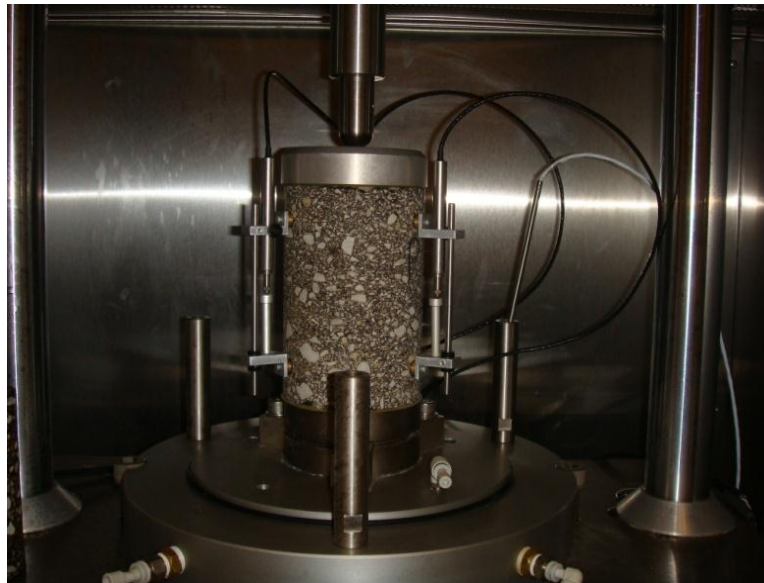
Figure 3.16 A Specimen with LVDTs mounted in the UTM-25kN
