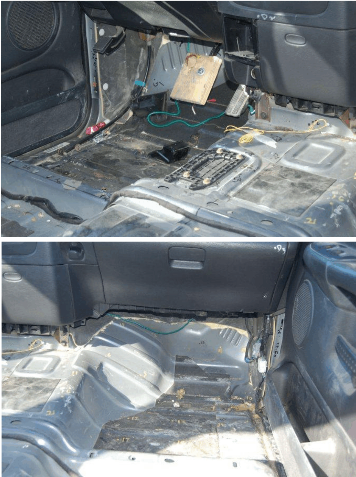
Figure 47. Occupant Compartment Damage, Test No. 4CMB-1
