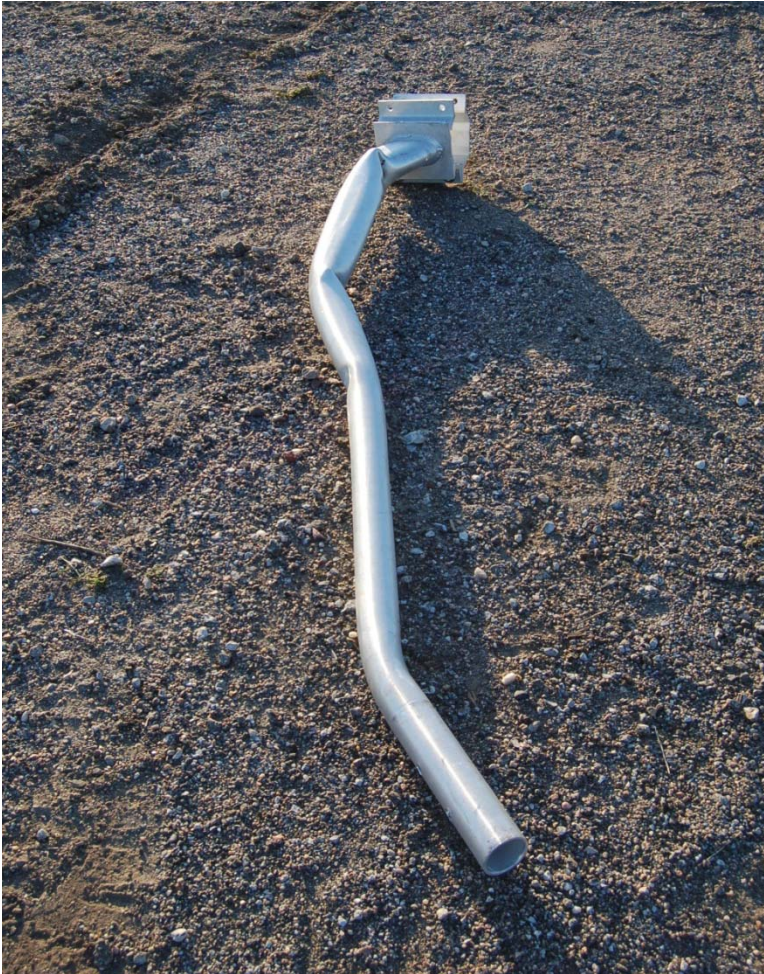
Figure 34. System Damage, Test No. BBC-2
