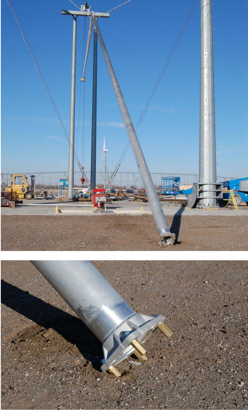
Figure 69. System Damage, Test No. BBC-7
