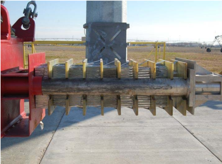
Figure 11. Crushable-Nose Pendulum Facility
