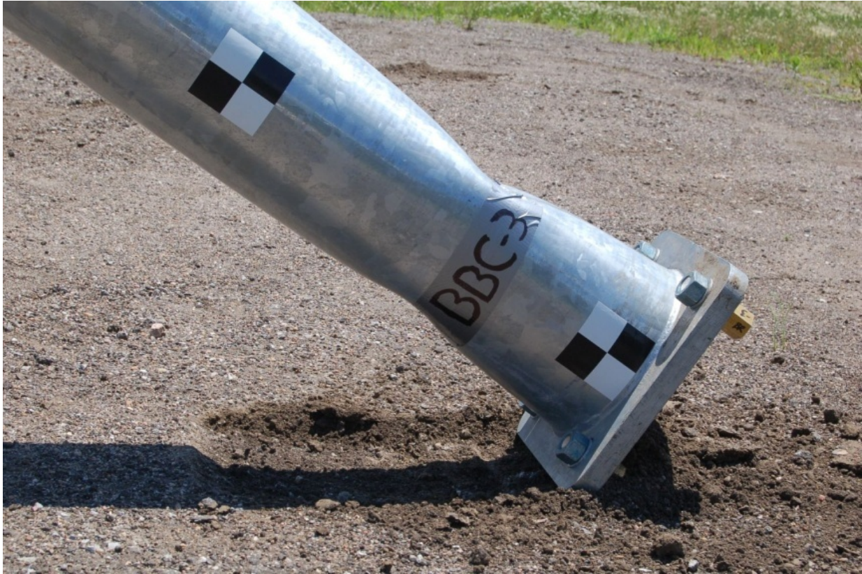
Figure 43. System Damage, Test No. BBC-3
