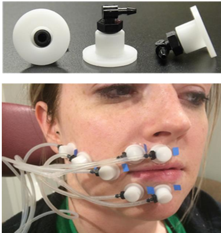
Figure 2.3 Pneumatic cells and array configuration
