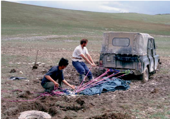
Fig. 13: Extracting YAZ jeep from mud hole, 6 July 1994. The tire burial technique is illustrated.
