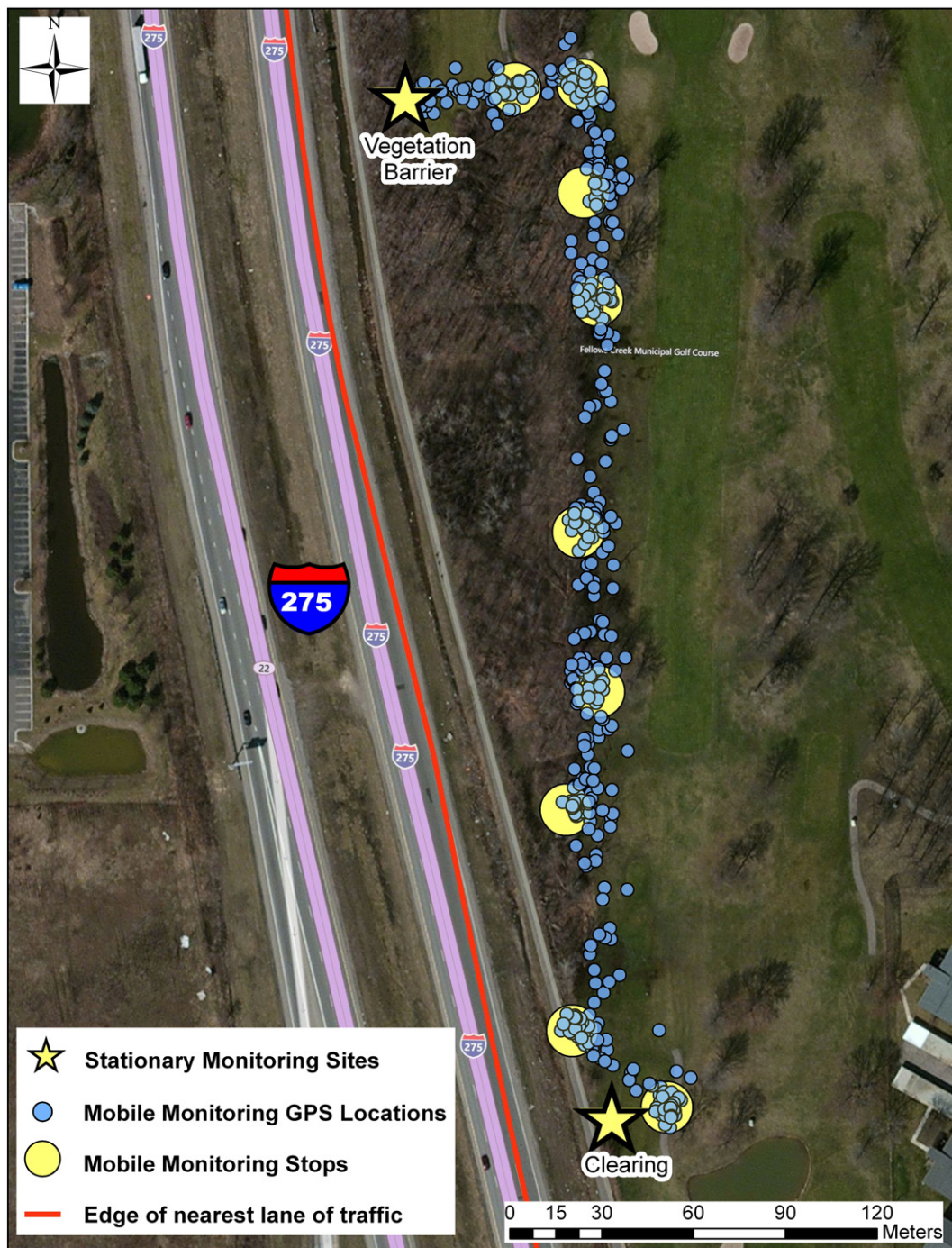
Fig. 1. Map of the study area in Detroit, Michigan showing the air monitoring locations. The star symbols indicate the locations of the fixed sites in a clearing (PS-C) and behind a tree stand (PS-T). The large yellow circles represent the intended sequential sampling stops, while the smaller, blue dots show the actual sampling locations during the mobile sampling campaigns. Changes in sampling locations from the intended sites were often a result of water hazards due to weather or use of the golf course.
