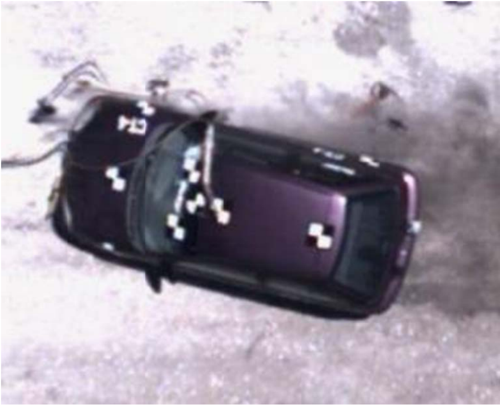
Figure 23. Geo Metro Overriding System Debris
