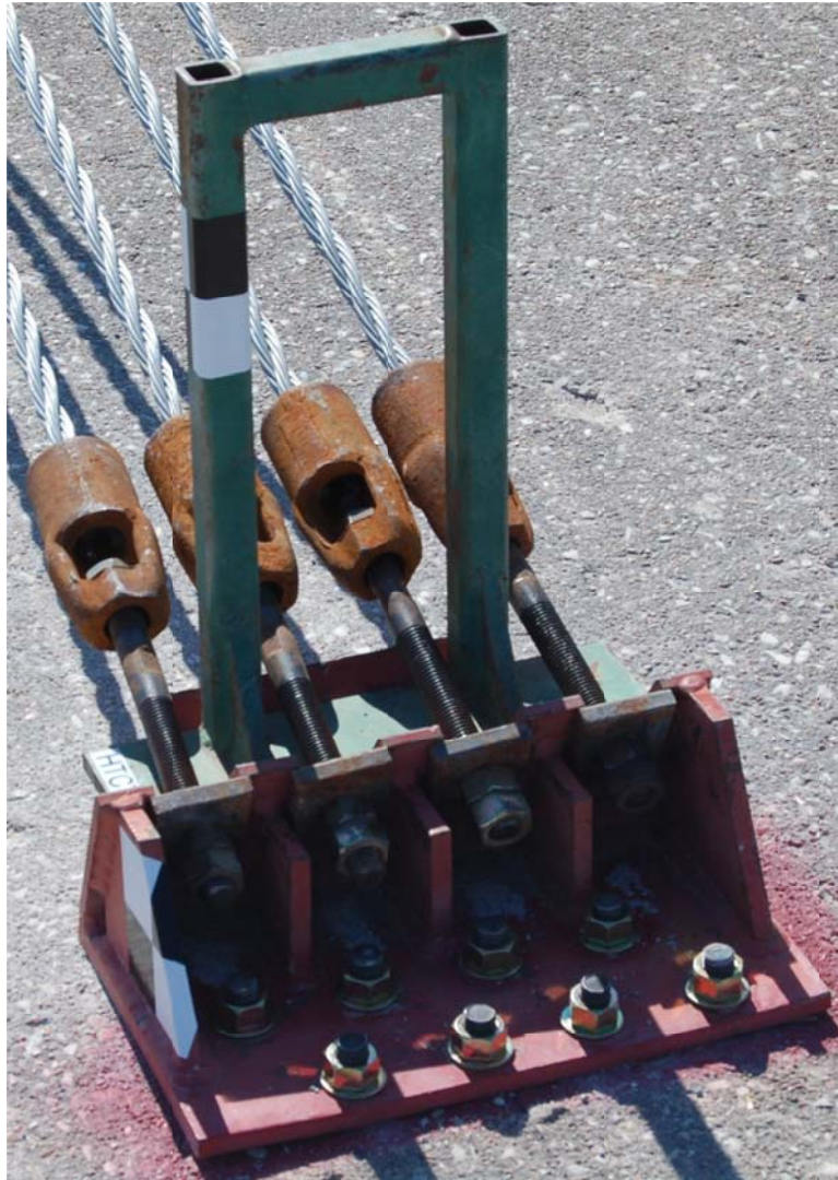
Figure 34. Cable Anchor Bracket and Finite Element Model
