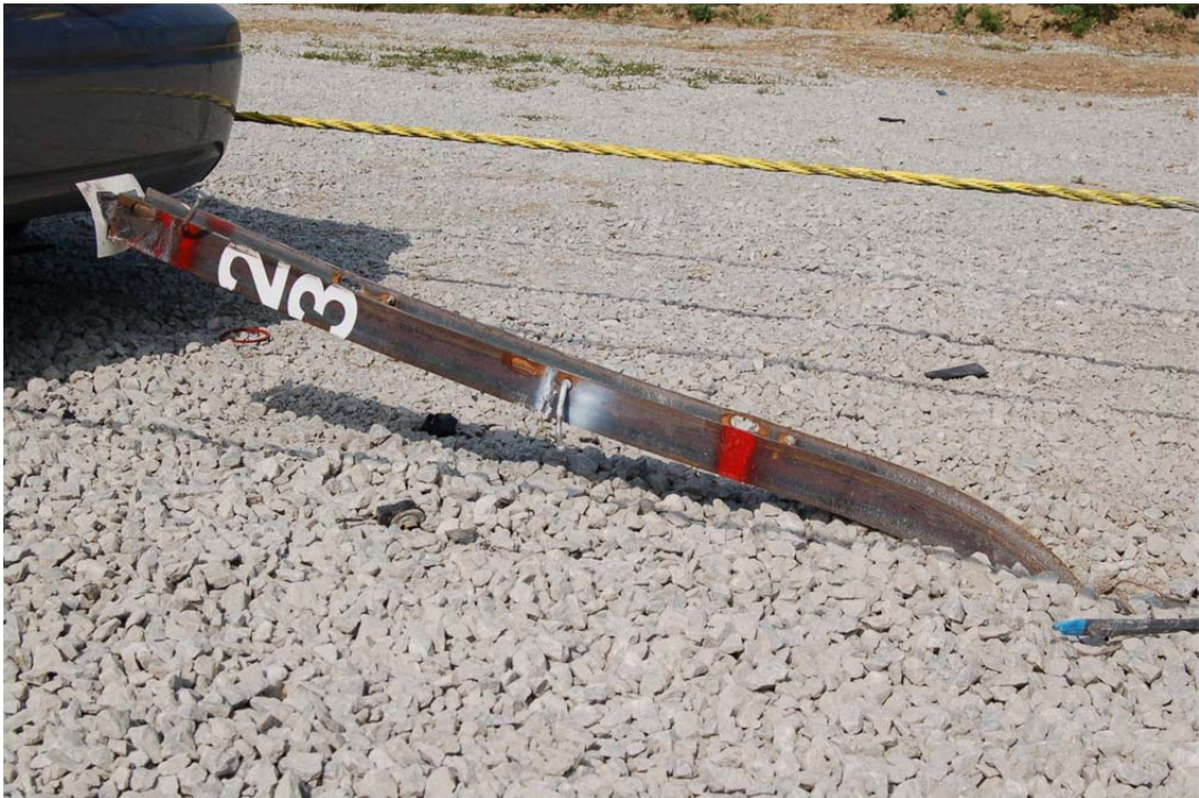
Figure 47. Post No. 23 Damage, Test No. 4CMBLT-1
