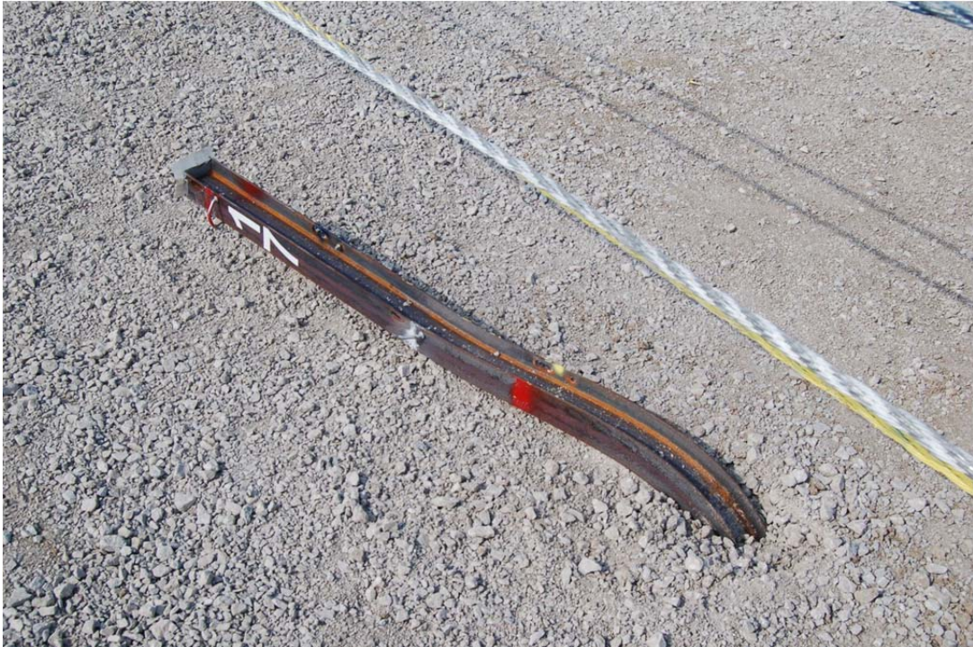
Figure 41. Post No. 17 Damage, Test No. 4CMBLT-1
