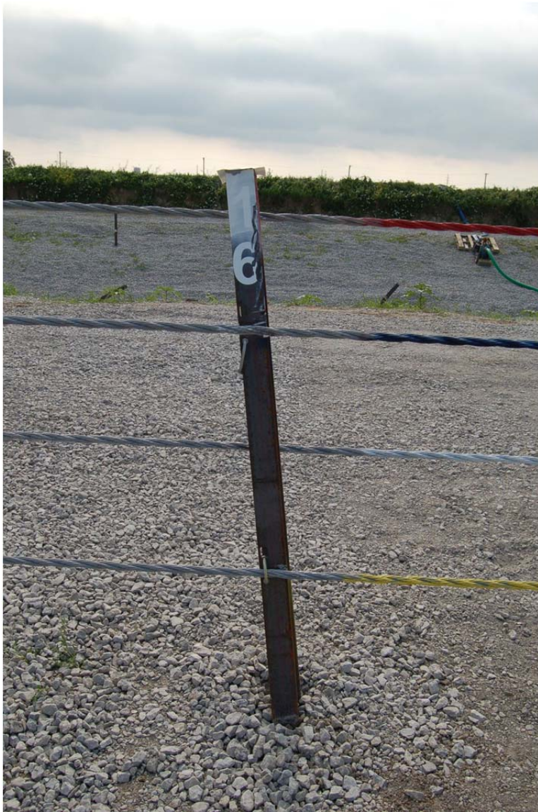
Figure 40. Post No. 16 Damage, Test No. 4CMBLT-1
