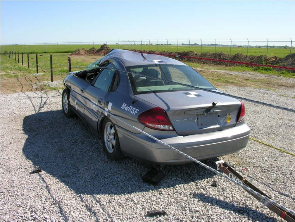
Figure 51. Vehicle Damage, Test No. 4CMBLT-1
