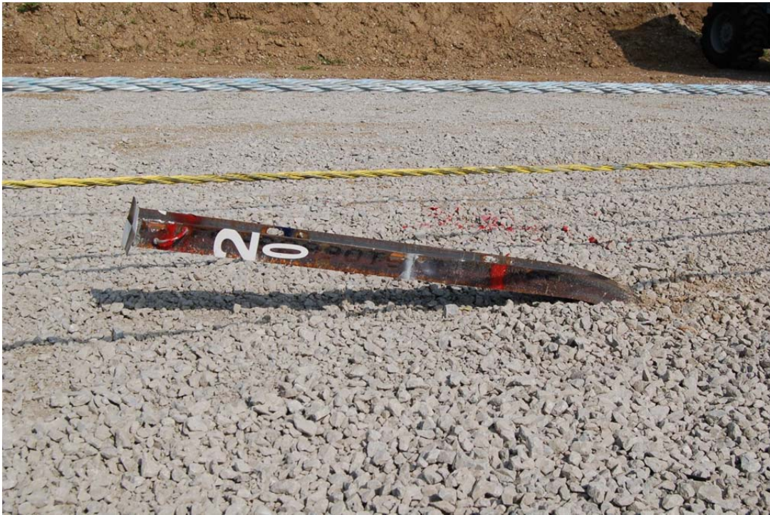
Figure 44. Post No. 20 Damage, Test No. 4CMBLT-1
