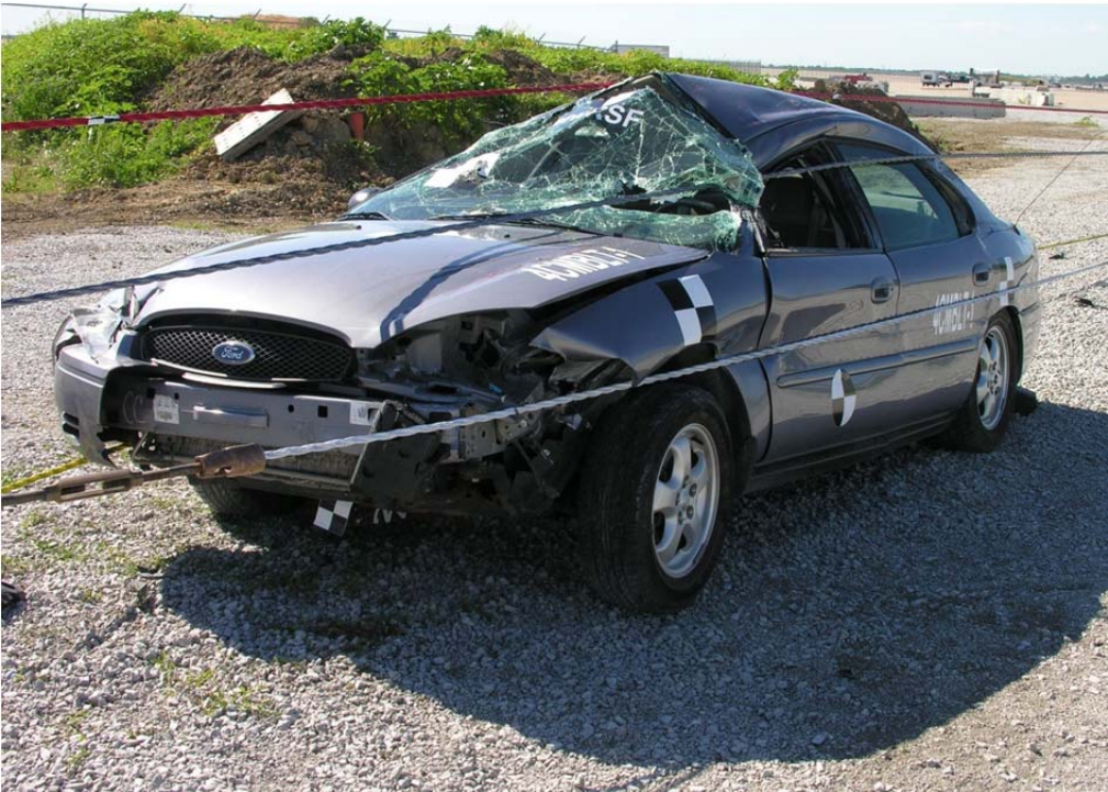
Figure 50. Vehicle Damage, Test No. 4CMBLT-1
