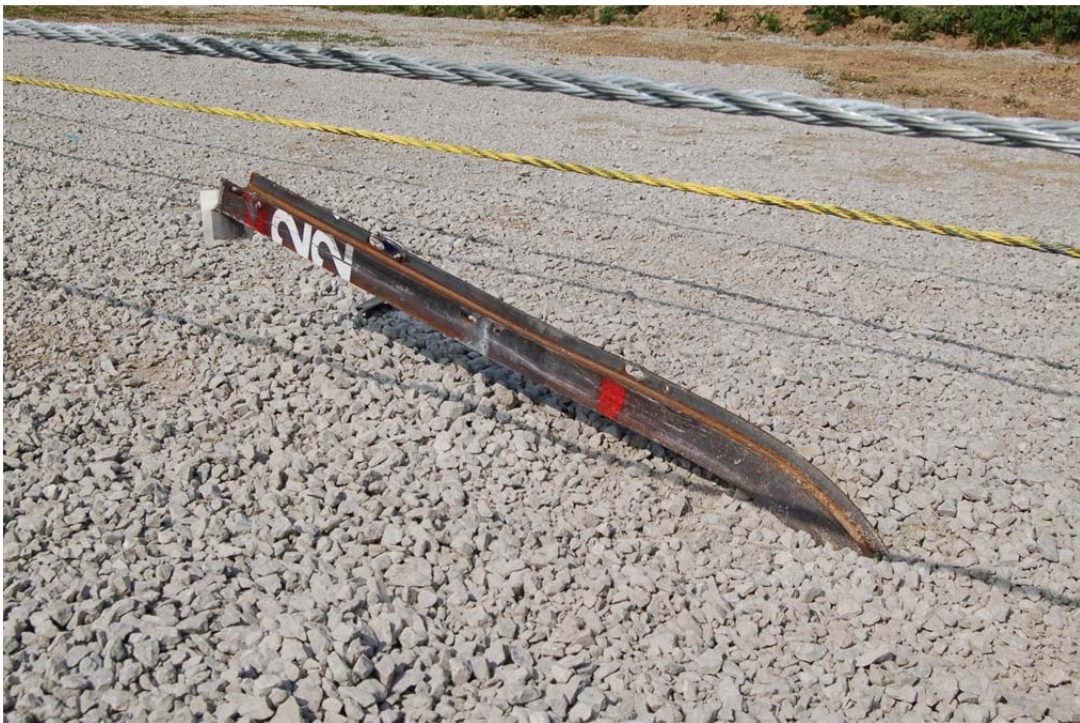
Figure 46. Post No. 22 Damage, Test No. 4CMBLT-1
