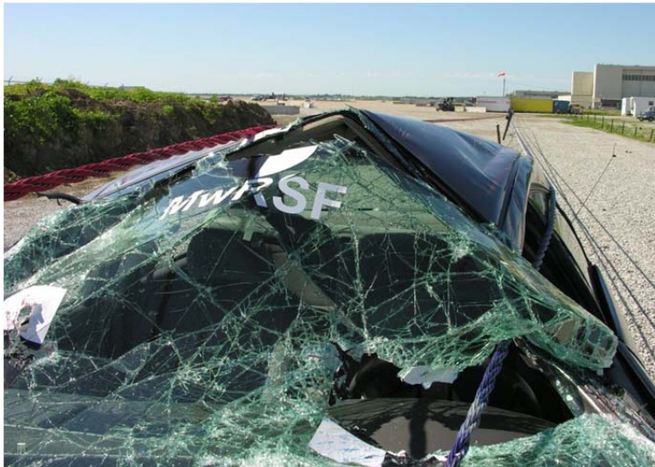
Figure 52. Vehicle Damage, Test No. 4CMBLT-1
