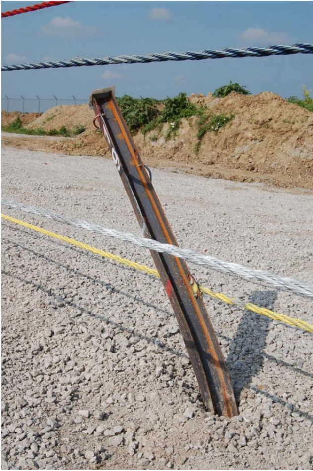
Figure 43. Post No. 19 Damage, Test No. 4CMBLT-1
