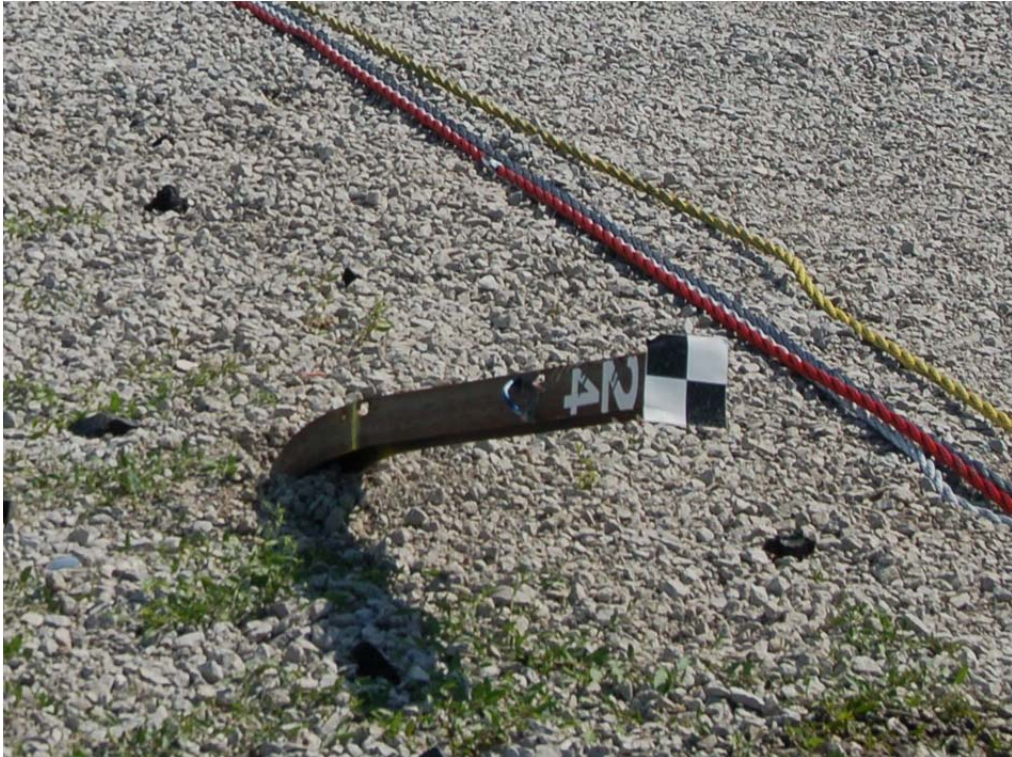
Figure 48. Post No. 24 Damage, Test No. 4CMBLT-1
