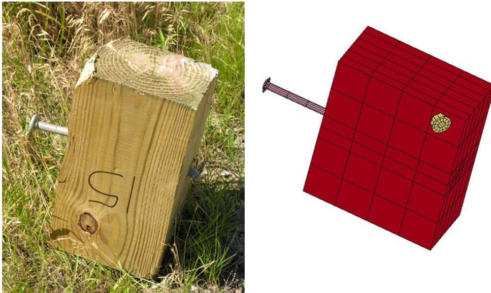
Figure 29. Blockout and Bolt from Test No. MGSMRH-1 and Simulation
