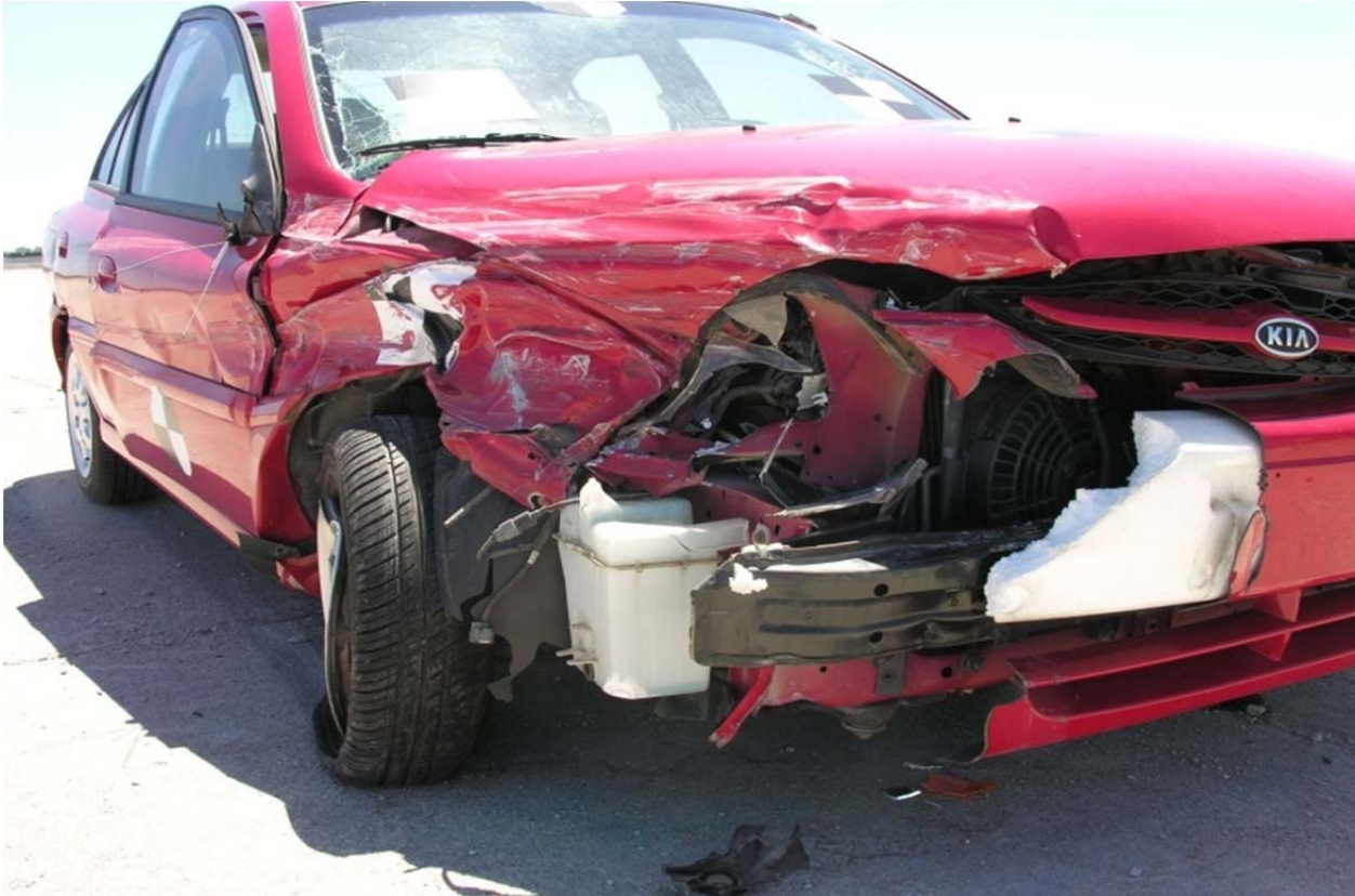
Figure 7. Test No. MGSMRH-1 Vehicle Damage
