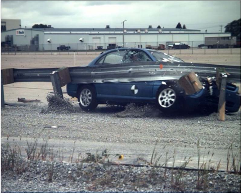
Figure 5. Test No. MGSMRH-2 Penetration
