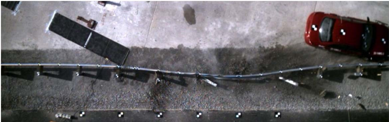
Figure 3. Vehicle Yaw Towards Barrier, test no. 2214MG-3
