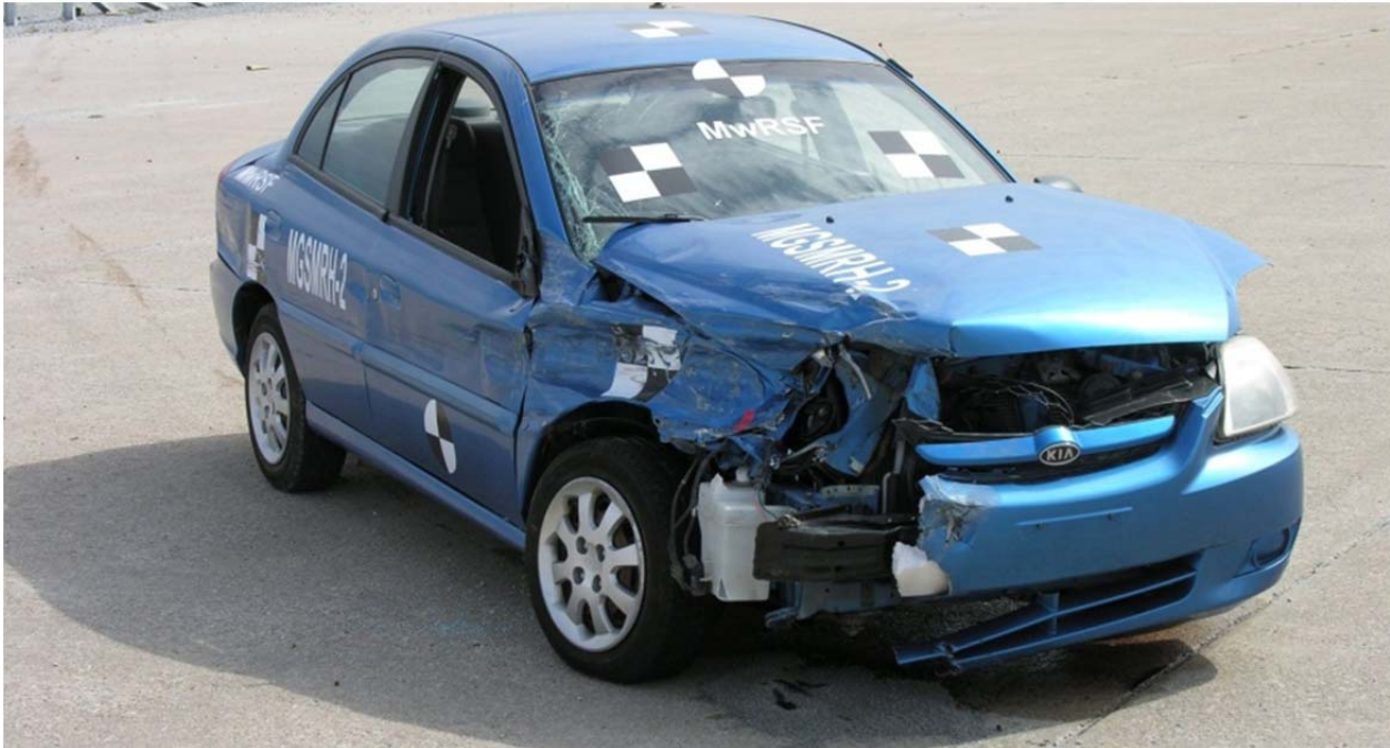
Figure 8. Test No. MGSMRH-2 Vehicle Damage
