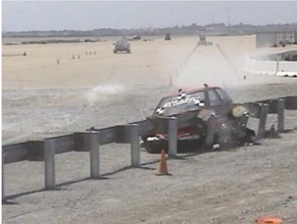
Figure 1. 820C Impact with MGS, test no. NPG-1
