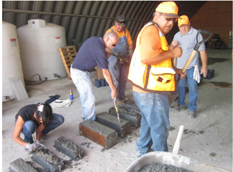
Figure 31. Casting of beams at the Concrete Ready Mix's Garage Facility
