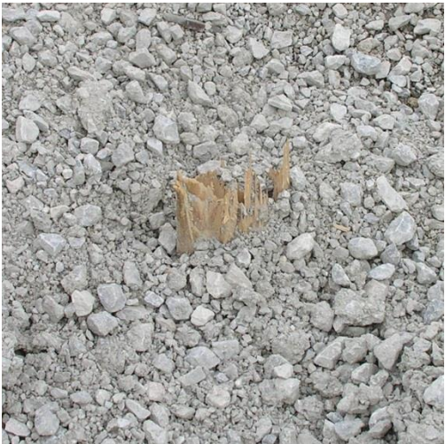
Figure 42. Post Nos. 15 and 16 Damage, Test No. MGSSYP-1
