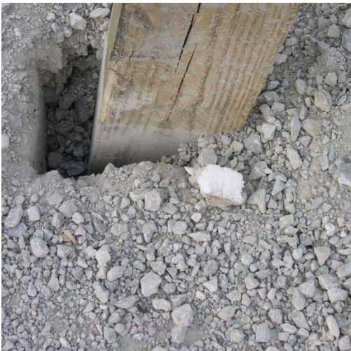
Figure 59. Post Nos. 17 and 18 Damage, Test No. MGSSYP-2
