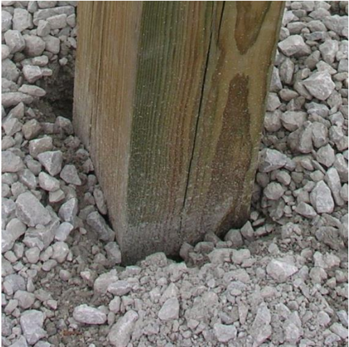
Figure 41. Post Nos. 13 and 14 Damage, Test No. MGSSYP-1
