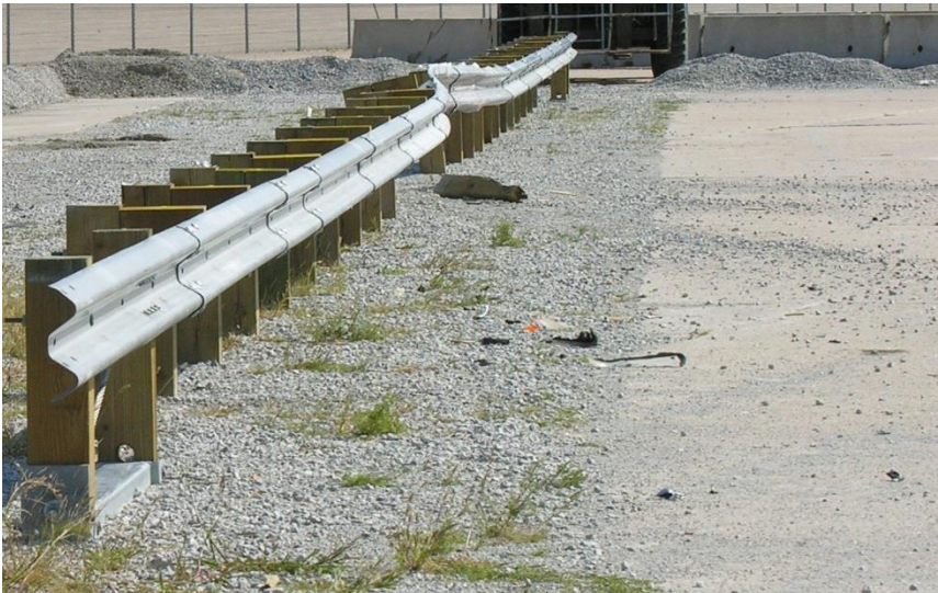
Figure 54. System Damage, Test No. MGSSYP-2
