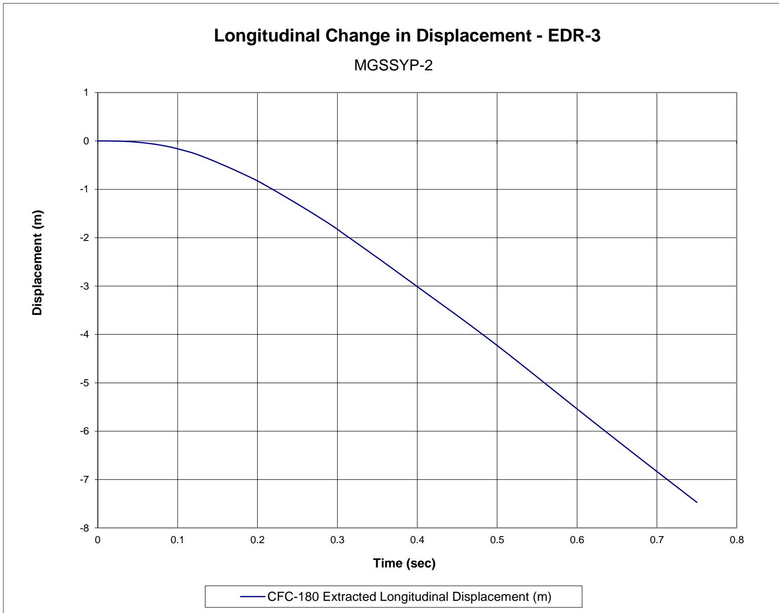
Figure F-11. Longitudinal Occupant Displacement (EDR-3), Test No. MGSSYP-2
