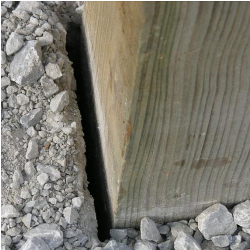
Figure 57. Post Nos. 13 and 14 Damage, Test No. MGSSYP-2
