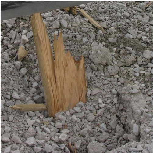
Figure 43. Post Nos. 17 and 18 Damage, Test No. MGSSYP-1
