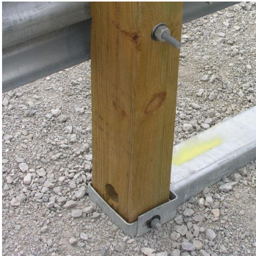
Figure 46. Downstream Anchor Damage, Test No. MGSSYP-1
