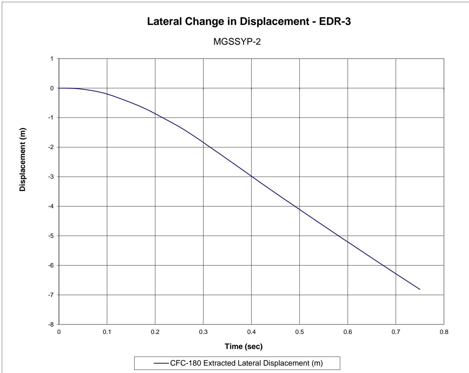
Figure F-14. Lateral Occupant Displacement (EDR-3), Test No. MGSSYP-2
