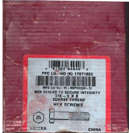
Figure A-49. 7/8 in. x 8 in. Hex Bolts, Test Nos. MGSSYP-1 and MGSSYP-2
