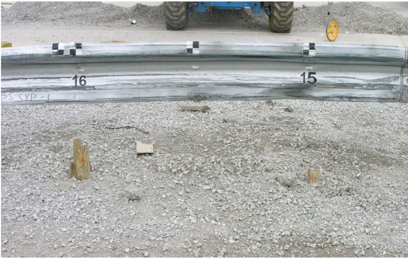
Figure 38. Rail Damage Between Post Nos. 13 and 18, Test No. MGSSYP-1
