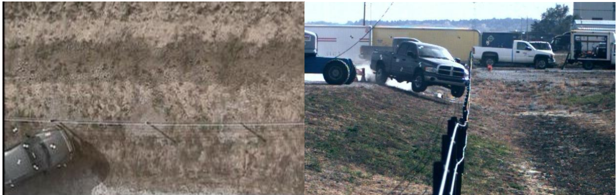
Figure 3.1 Vehicle-Cable Impact of Test 4CMB-1
