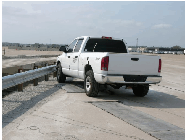
Figure 31. Impact Location, Test No. MGS221-1
