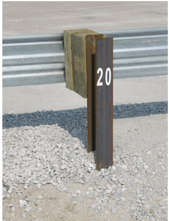
Figure 22. MGS Installed Adjacent to a 2:1 Fill Slope, Test No. MGS221-1
