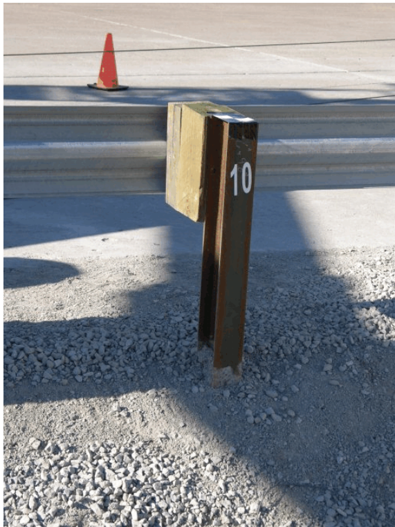
Figure 49. MGS Installed Adjacent to a 2:1 Fill Slope, Test No. MGS221-2
