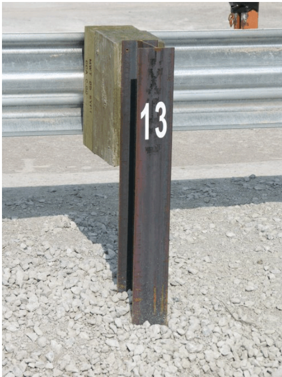
Figure 22. MGS Installed Adjacent to a 2:1 Fill Slope, Test No. MGS221-1
