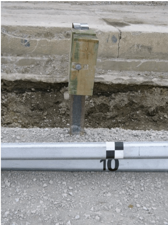
Figure 60. Post Nos. 9 through 12 Damage, Test No. MGS221-2
