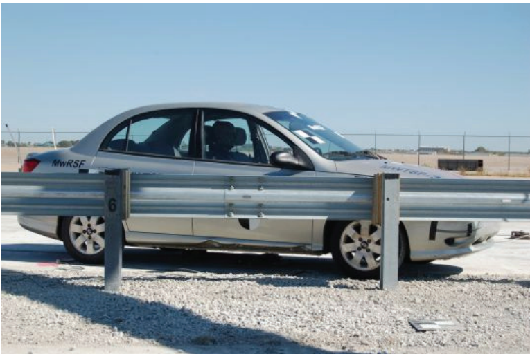
Figure 83. Impact Location. Test No. MWTSP-3
