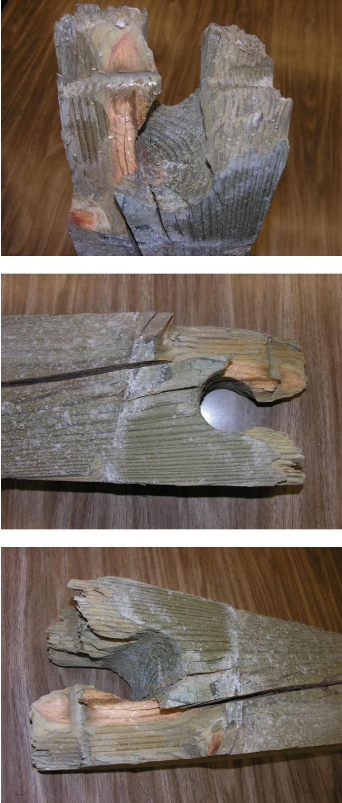
Figure 61. Anchorage Post No. 1 Damage, Test No. MWTSP-1
