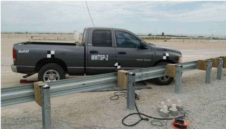
Figure 68. Impact Location, Test No. MWTSP-2
