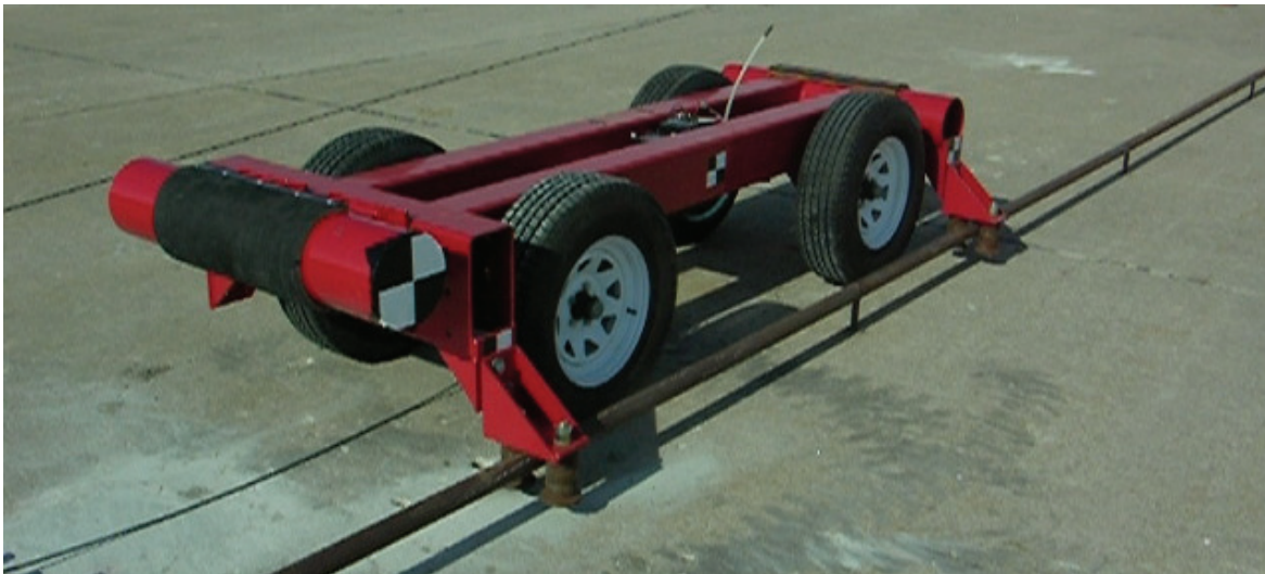
Figure 2. Rigid Frame Bogie on Guidance Track
