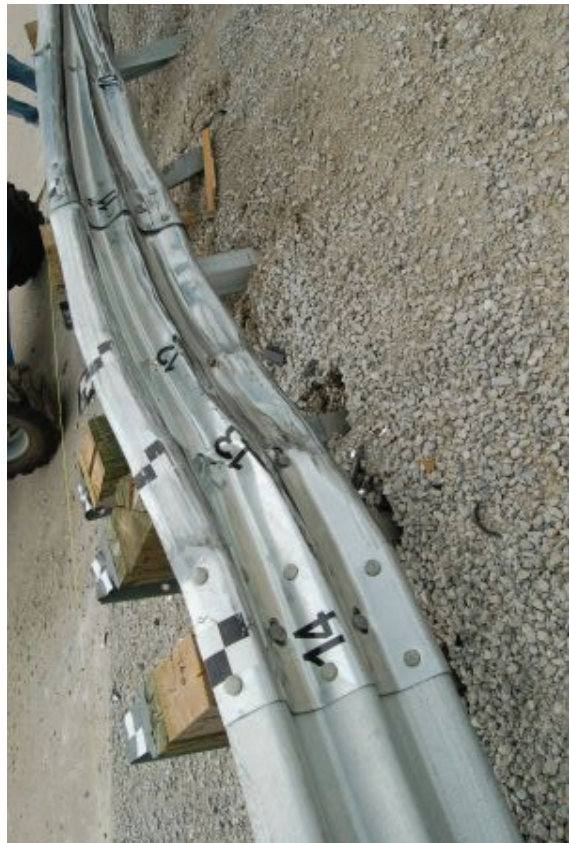
Figure 74. Post Nos. 12 through 14 Damage, Test No. MWTSP-2
