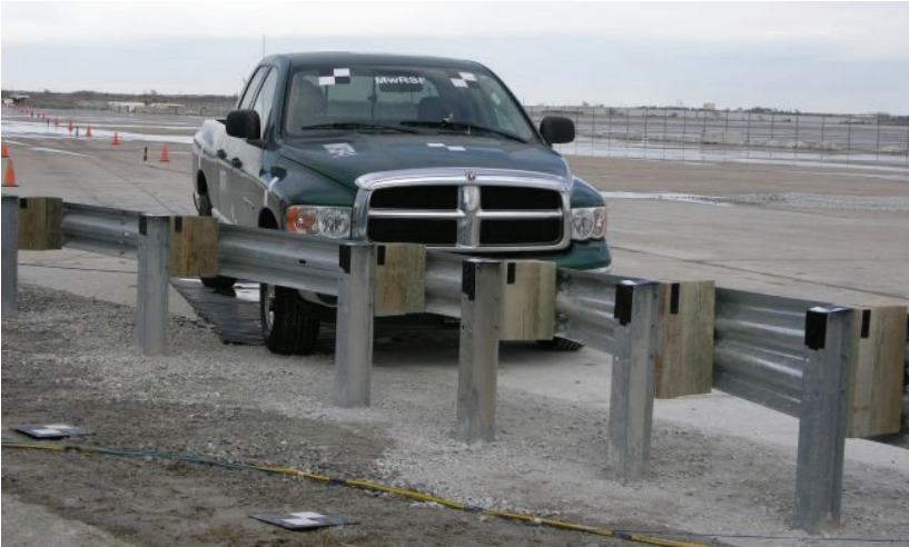
Figure 53. Impact Location, Test No. MWTSP-1
