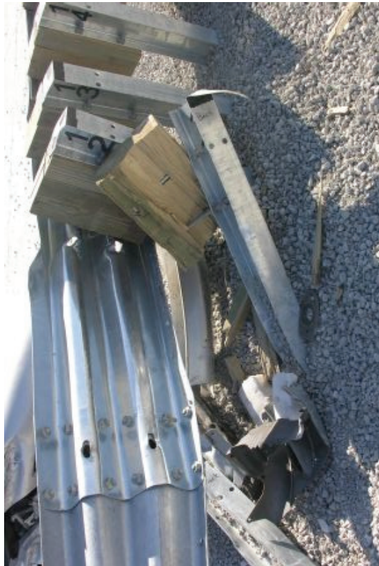
Figure 88. Post Nos. 12 through 14 Damage, Test No. MWTSP-3
