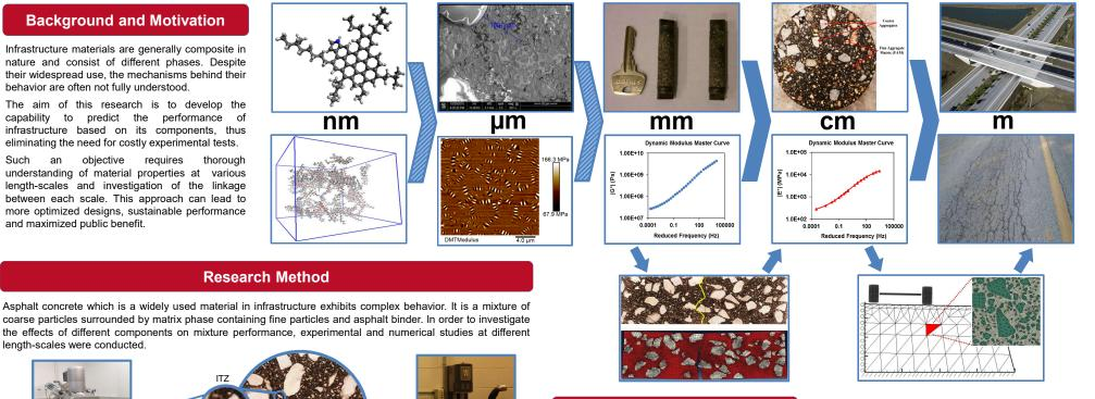
coarse particles surrounded by matrix phase containing fine particles and asphalt binder. In order to investigate the effects of different components on mixture performance, experimental and numerical studies at different length-scales were conducted.
